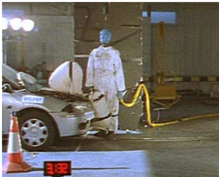
Figure 8. Actual test undertaken by TRL Ltd showing external pedestrian protection device concepts.
