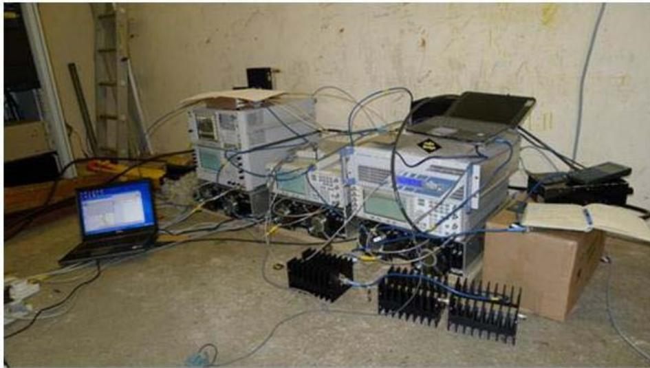
**Figure 3.5: LTE transmission equipment at Council Office site**
