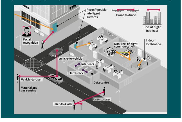
Figure 22: Examples of applications for THz communication and sensing. Source: Ofcom, based on [Sarieddeen2020].
