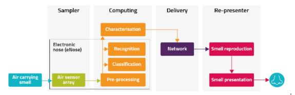
*Figure 7: Architecture for transmission of scents over a communication network. Source: [Wen2018].*
