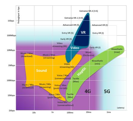
Figure 9: Estimate of minimum throughput and reciprocal latency requirements for delivery of each form of sensory communications<sup>18</sup>. Source: Ofcom.
