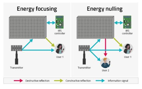
Figure 18: Examples of ways of using intelligent reflecting surfaces (IRS) for energy focusing towards a user or to nullify or reduce the interference towards another user. Source: Ofcom and Emil Björnson.
