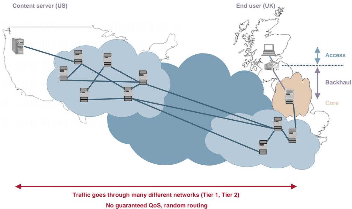
Figure 4.1: End-to-end traffic routing via the public Internet [Source: Analysys Mason]
