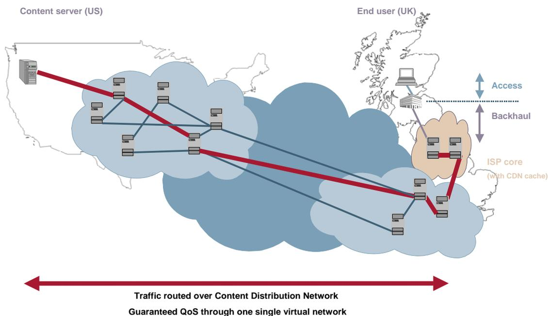
Figure 1.3: End-to-end traffic routing using a content distribution network [Source: Analysys Mason]
