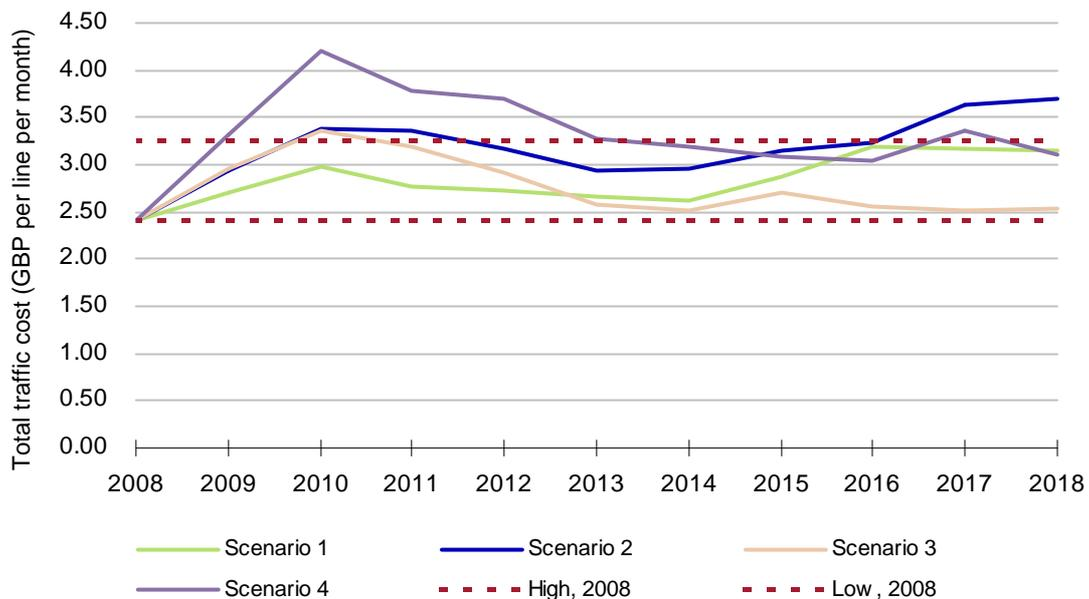
Figure 6.30: Overview of the total monthly cost per line when deploying all technical solutions for Scenarios 1 to 4 for a bitstream-based service provider [Source: Analysys Mason]
