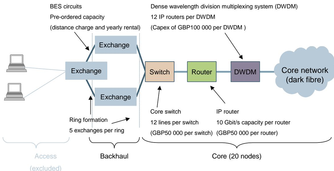
Figure 6.3: LLU architecture for an alternative operator [Source: Analysys Mason]
