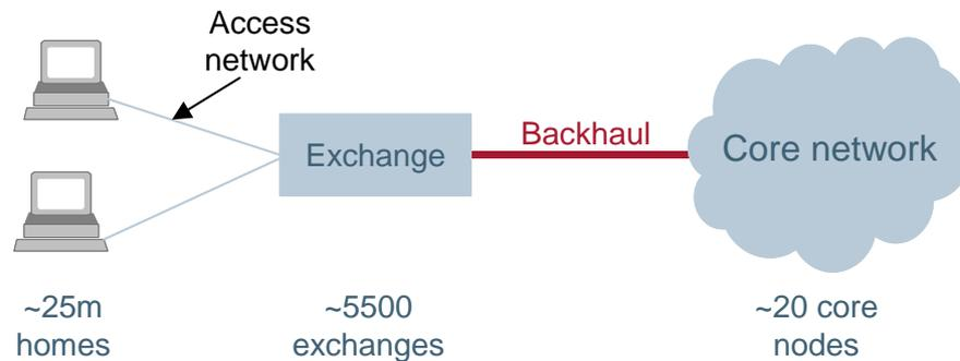
Figure 4.3: Illustration of access, backhaul and core networks [Source: Analysys Mason]
