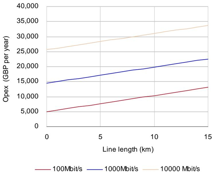
Figure 6.5: Yearly cost per BES line with different bandwidths
