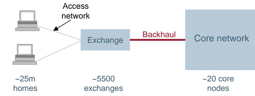
Figure 1.4: Illustration of access, backhaul and core networks [Source: Analysys Mason]
