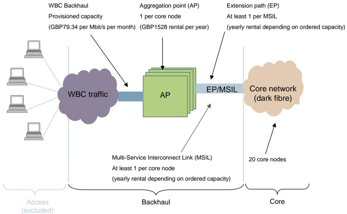
Figure 6.11: Schematic illustration of WBC setup and cost components [Source: BT Wholesale]
