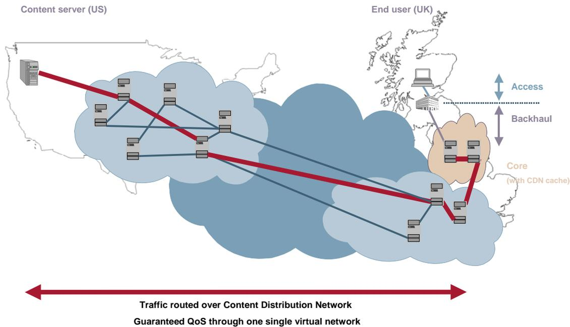
Figure 4.2: End-to-end traffic routing using a CDN [Source: Analysys Mason]
