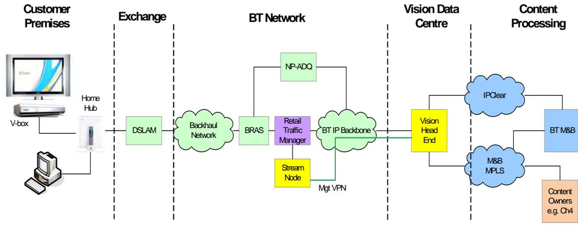
Figure C.19: Network diagram for BT Vision [Source: Analysys Mason]
