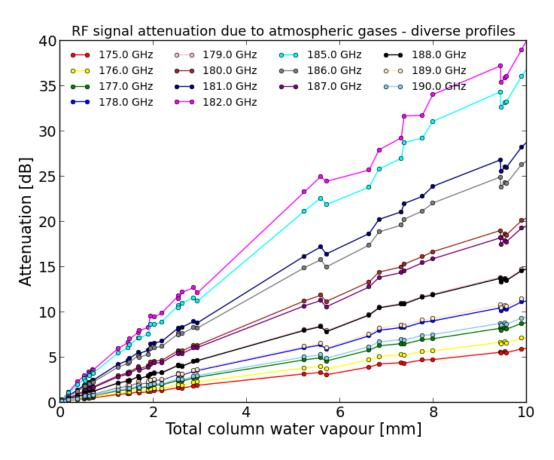
Figure 5: Attenuation as a function of TCWV
