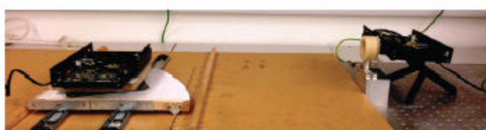
Figure 6-9 Practical experimental setup including transmitter on the right and receiver on the left.
