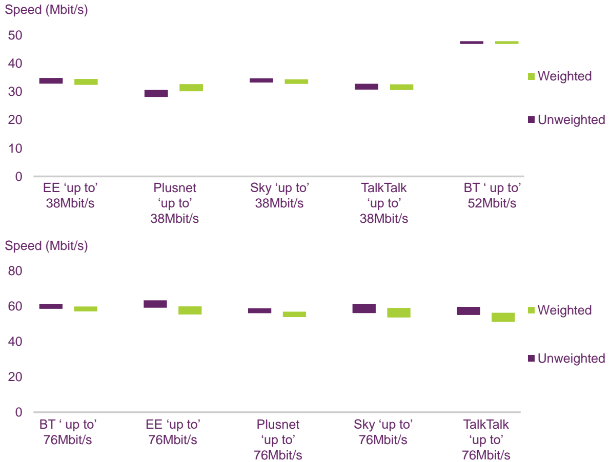
Figure 2.12: Peak-time (8pm to 10pm) download speeds for FTTC ISP packages, weighted and unweighted figures: November 2016
