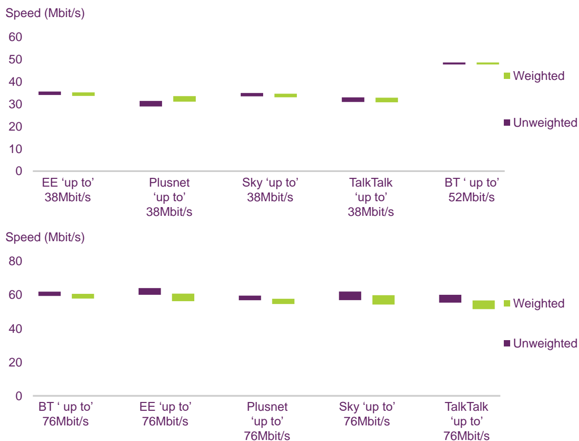
Figure 2.11: Average download speeds for FTTC ISP packages, weighted and unweighted figures: November 2016
