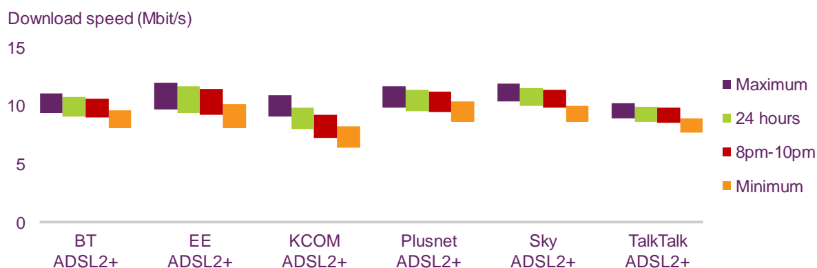
Figure 26: Maximum, average, peak-time and minimum download speeds for ADSL2+ ISP packages, and significant differences, to a 95% level of confidence
