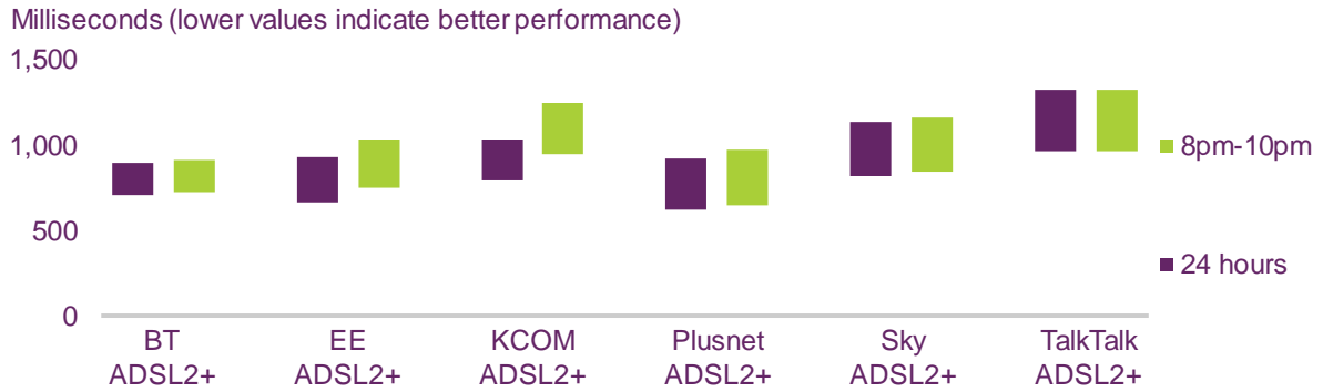
Figure 40: Average and peak-time loading of web pages for ADSL2+ ISP packages and significant differences, to a 95% level of confidence: November 2016
