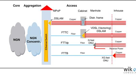
MPoP: Metropolitan Point of Presence, also called ODF location (Optical Distribution Frame), is equal or comparable to a Local Exchange
