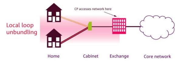
**Local Exchange / Exchange:** The local exchange refers both to a building and the equipment within it. It is the location at which local access network lines (both copper and fibre) will end, and will be connected to the relevant equipment. Exchanges may house DLEs and concentrators for voice services; DSLAMs for broadband; or MSANs for both voice and broadband in an NGN. In the BT network there are around 5,500 exchange buildings across the UK.
