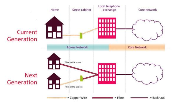
**Next Generation Networks (NGN):** A 'Next Generation Network' is generally understood to refer to an IP network capable of being used for both voice and data, and in which there is some control over quality of service. The key features of an NGN are that it is a packetbased, multi-service network, which has a clear separation of transport and control, and where the control functions may reside on a physically separate network.
