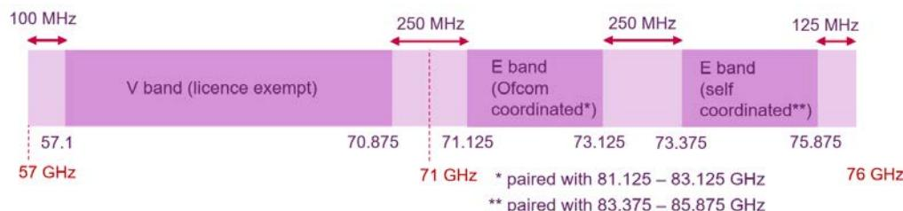
Figure 3: Frequency separation below 71 GHz
