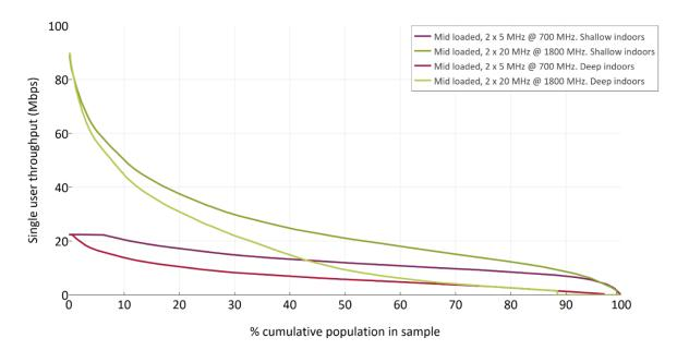
A6.105 2 x 20 MHz of 1800 MHz provides higher SUT than 2 x 5 MHz of 700 MHz due to the bandwidth available being four times greater. In this case the difference gap is bigger than that when comparing with 2 x 10 MHz of 700 MHz, which leads to fewer locations getting the same levels of SUT.
