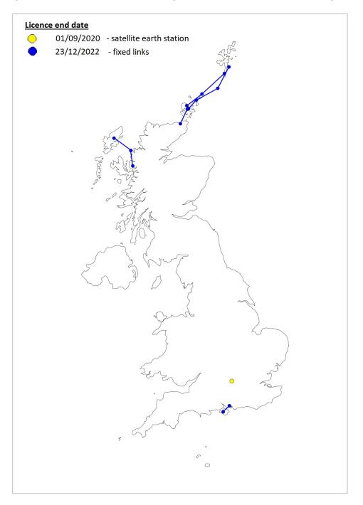
A8.6 There is one link operating between the Isle of Wight and Portsmouth which could potentially constrain early mobile deployments. This link operates a 30 MHz carrier centred at 3740 MHz. Below we describe the approach we used to estimate the scale of the likely impact of the protection of this link on the deployment of mobile base stations in the interim period.
