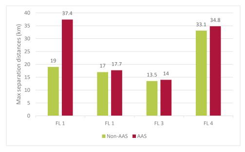
A8.65 The maximum interfering distances shown in Tables A8.9 and A8.10 are larger than those we observed for satellite earth stations. This is because the fixed link antennas cannot benefit from elevation angle like satellite earth stations can to reject terrestrial interfering
