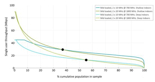
Figure A6.9 SUT distribution curves, shallow and deep indoor locations in the mid densely populated area (2 x 10 MHz of 700 MHz and 2 x 20 MHz of 1800 MHz)
