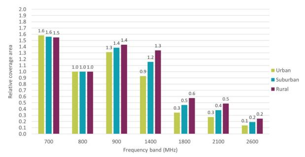
A6.83 These results show that the 1400 MHz potential coverage is estimated to be greater than the 800 MHz potential coverage in all cases, with the exception of the coverage in deep indoor locations in urban environments, which is estimated to be approximately 10% less. On the other hand, the potential coverage from 1800 MHz and higher bands is estimated to be significantly lower than from the 700 MHz, 800 MHz, 900 MHz and 1400 MHz bands.
