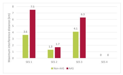
Figure A8.5: Chart of the satellite earth station worst case area analysis results using long term protection criteria
