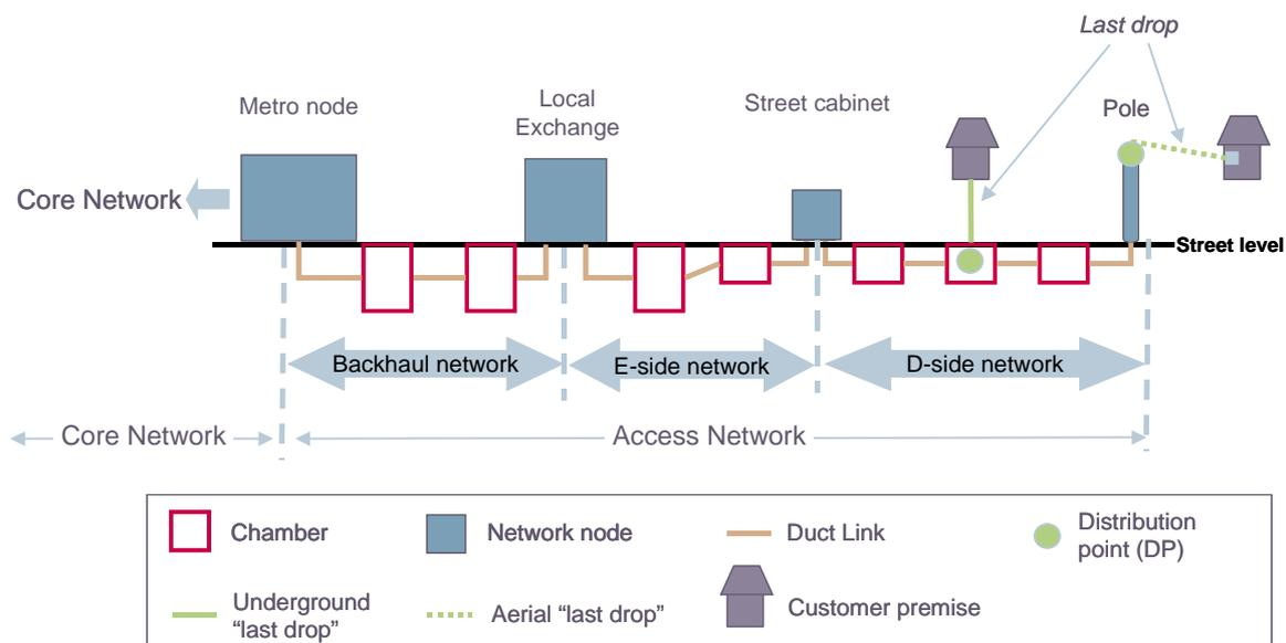
Figure 3.1: Diagrammatic representation of UK incumbent network [Source: Analysys Mason]
