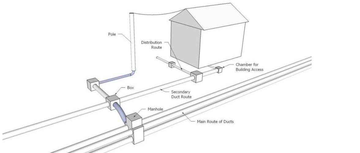
Figure 3.2: Tree and branch configuration of the access network [Source: Analysys Mason]
