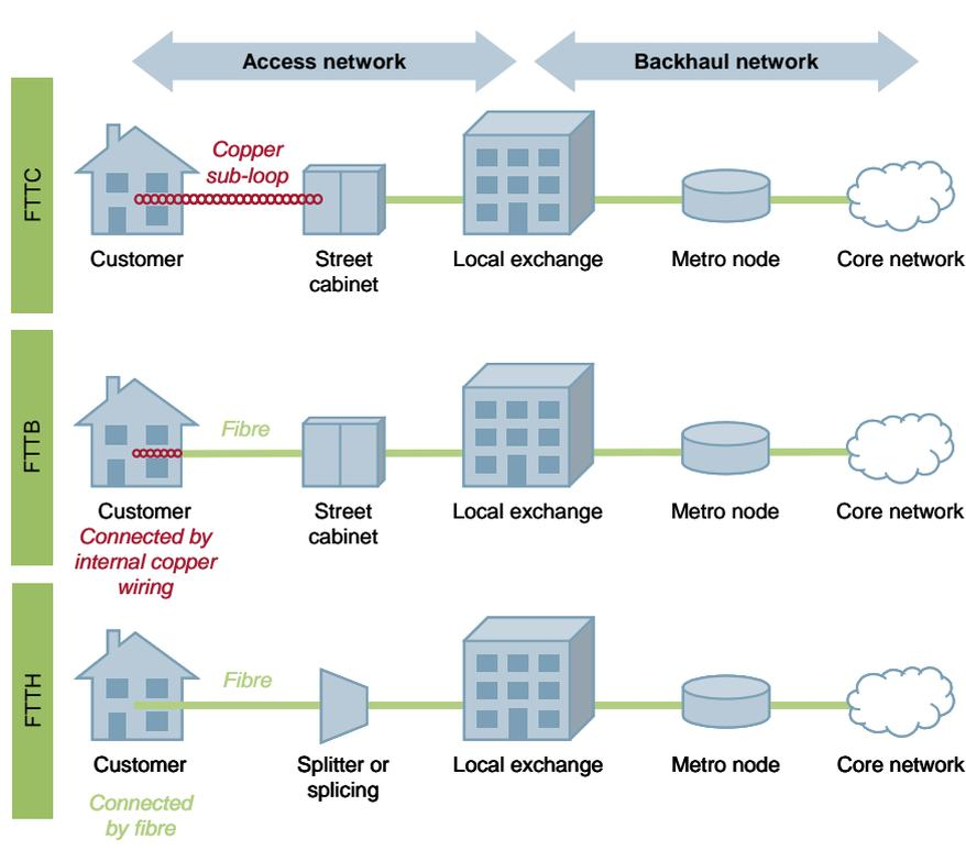
Figure 3.9: FTTx architectures [Source: Analysys Mason]
