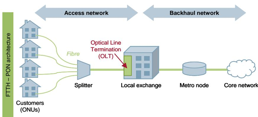
Figure 3.12: Passive optical network architecture [Source: Analysys Mason]
