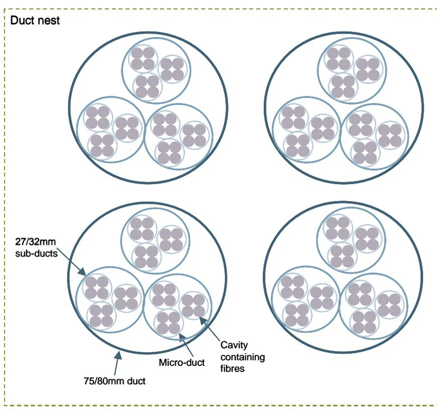
Figure 4.5: Duct nest showing potential layers of ducting within a duct nest [Source: Analysys Mason]
