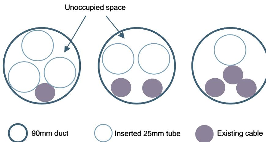
Figure 3.7: Examples of the use of sub-duct [Source: Analysys Mason]
