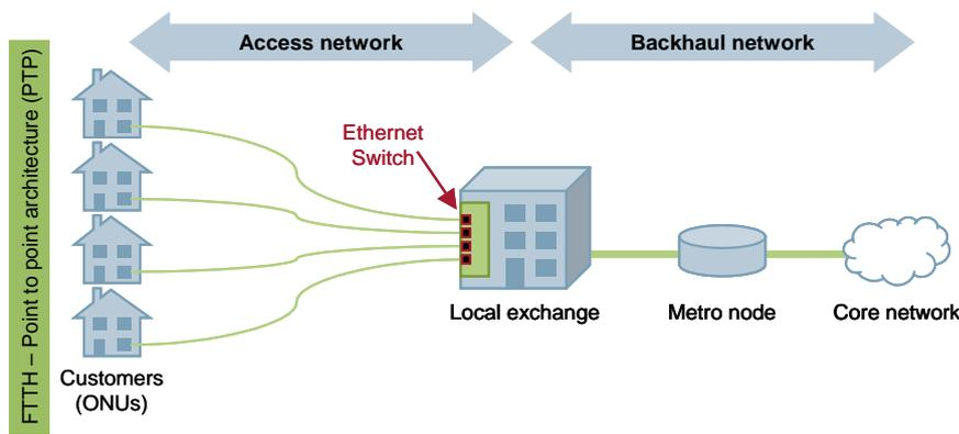
Figure 3.11: Typical PTP architecture [Source: Analysys Mason]
