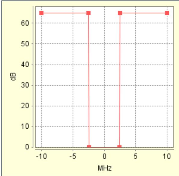
Figure 33. LTE receiver blocking mask
