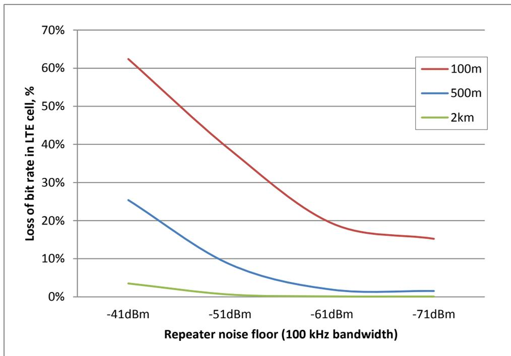
Figure 21. Interference to LTE cell vs repeater noise floor
