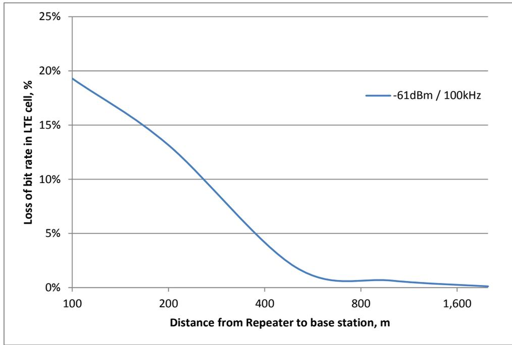
Figure 20. Interference to LTE cell vs repeater distance
