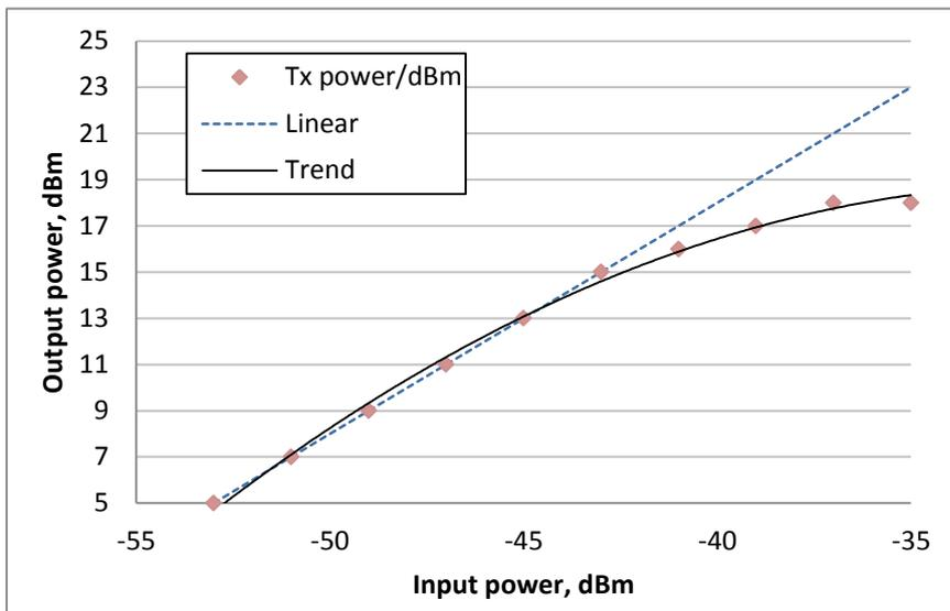
Figure 23. 900UL gain compression
