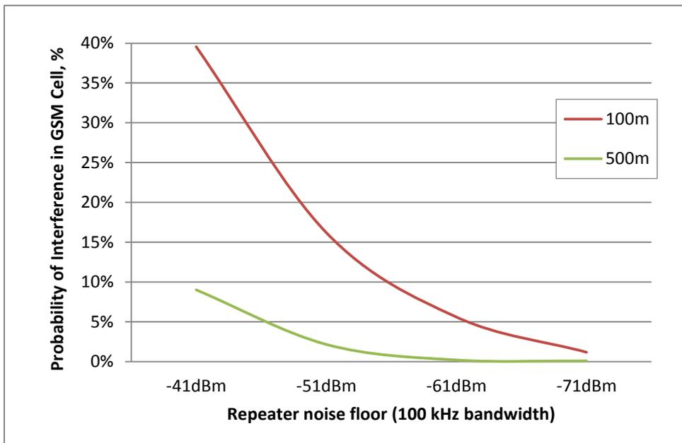
Figure 17. Interference to GSM cell vs repeater noise floor
