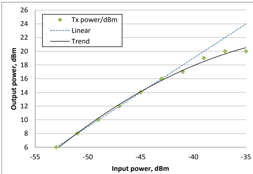
Figure 25. 1800UL gain compression
