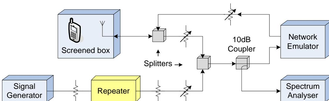
**Figure 6. Measurement of effect on networks**
