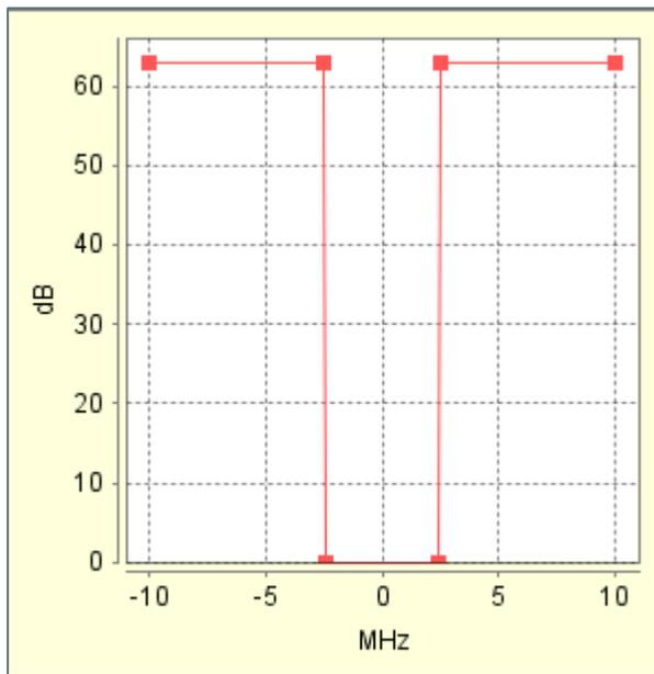
Figure 32. 3G receiver blocking mask
