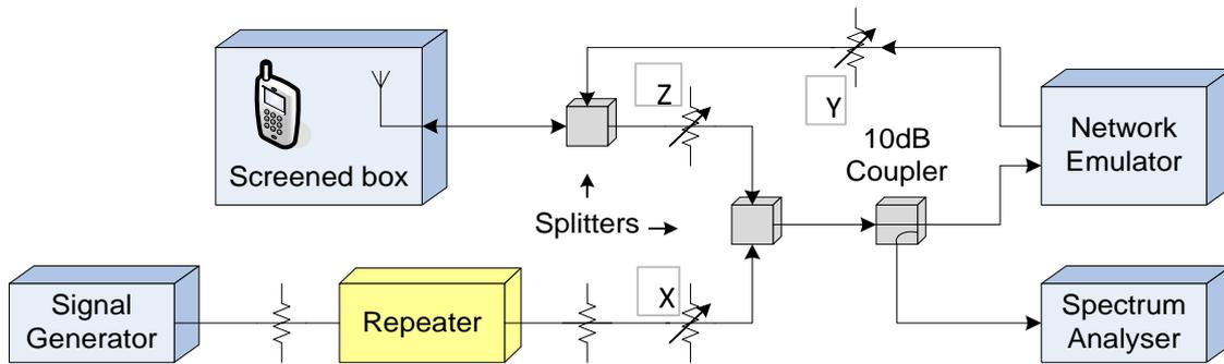
**Figure 26. Network emulation test configuration**
