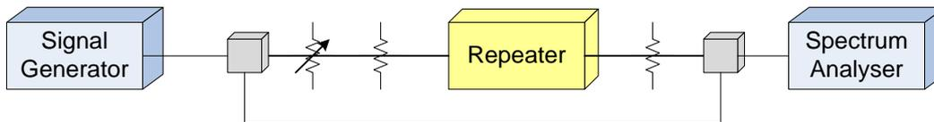
**Figure 5. Measurement of RF characteristics**
