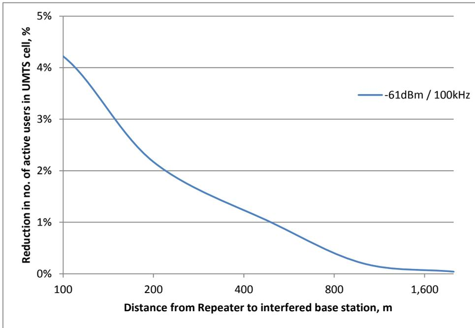
Figure 18. Interference to 3G cell vs repeater distance
