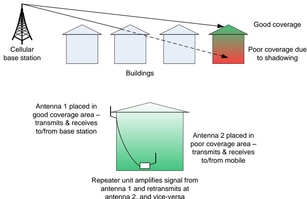
**Figure 1. Mobile network repeater**
