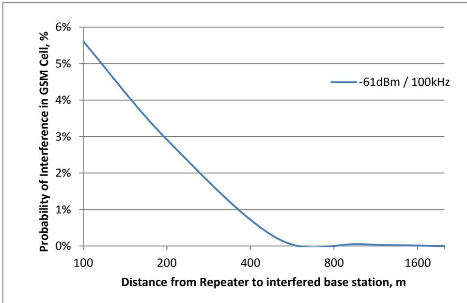
Figure 16. Interference to GSM cell vs repeater distance
