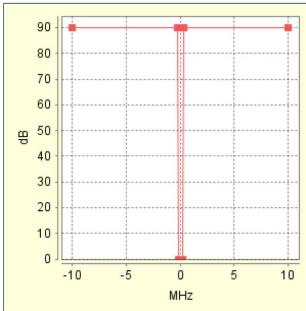
Figure 31. GSM receiver blocking mask
