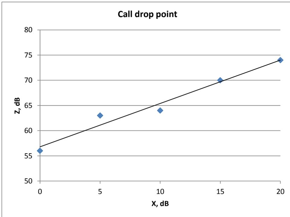
**Figure 27. Attenuator settings for GSM interference**
