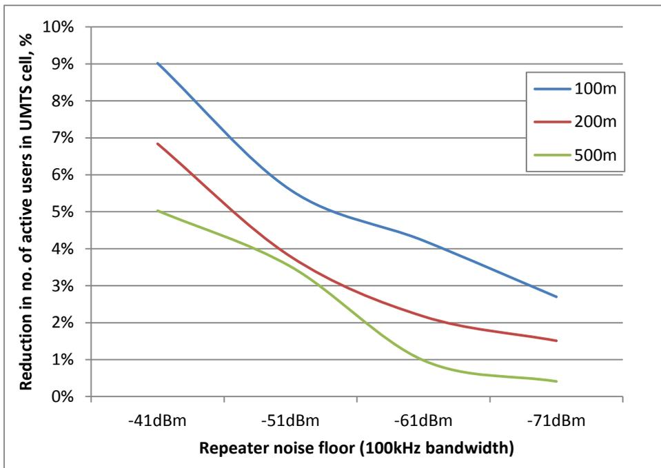
Figure 19. Interference to 3G cell vs repeater noise floor
