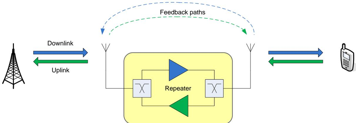
**Figure 4. Feedback paths around a repeater**
