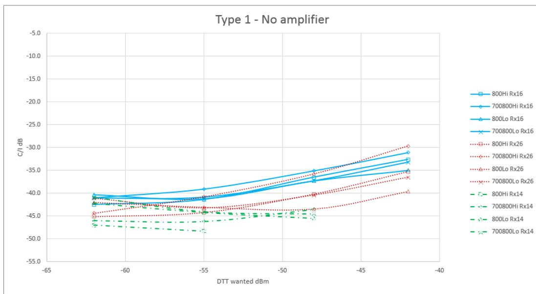
**Figure A4.5: C/I ratios for installation with a poor pre-amplifier**
