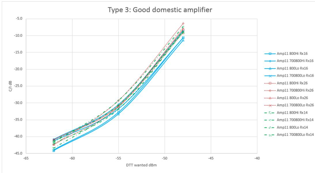
**Figure A4.9: C/I ratios for installation with a poor launch amplifier**
