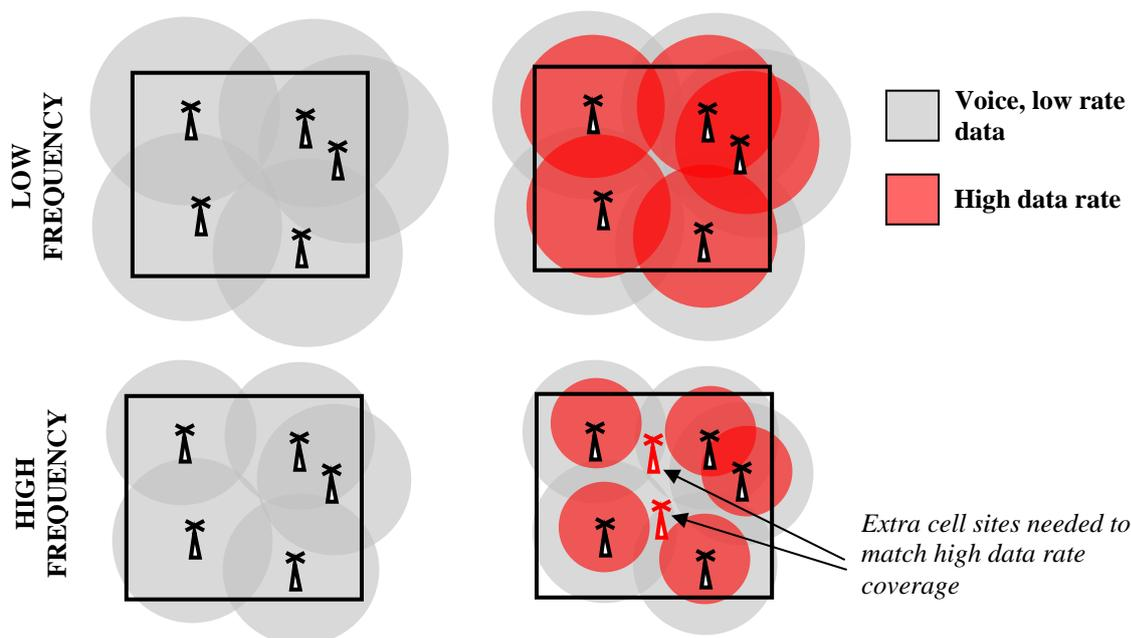
*With similar cell site distribution basic services can be offered with similar coverage at both low and high frequency*
