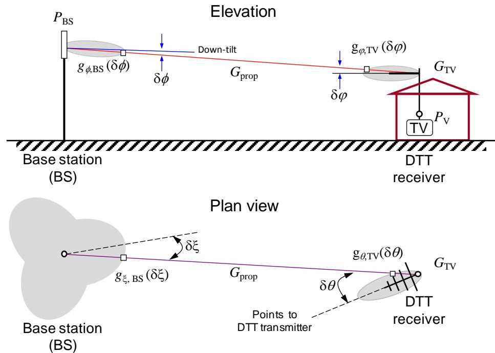
Figure 6. Geometry of base station to TV radio link.
