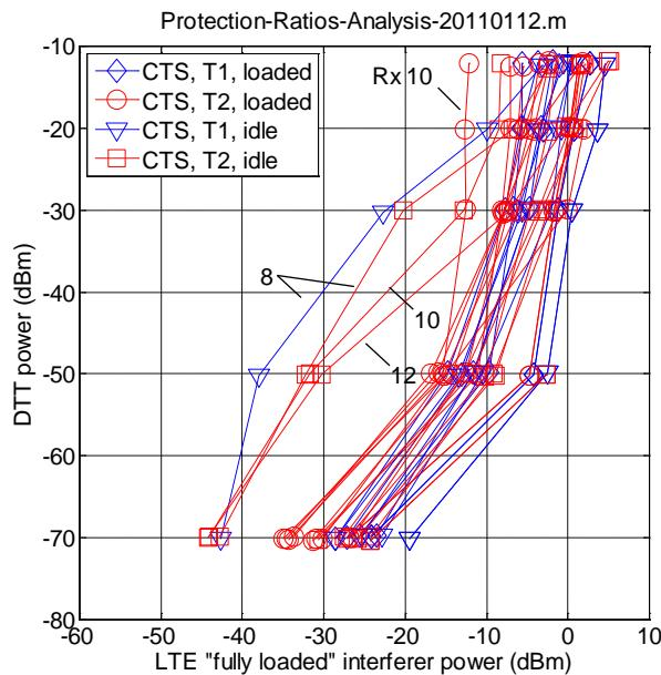
Figure 60. ERA raw protection ratio measurements (channel 60).
