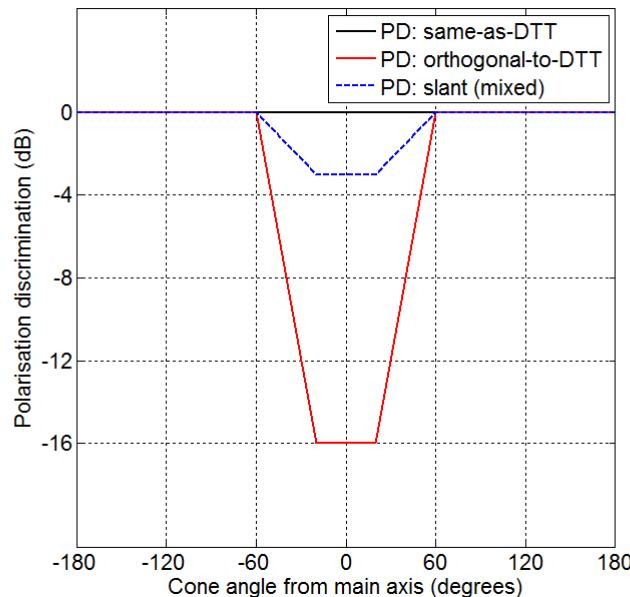
Figure 21. TV aerial polarisation discrimination as a function of cone angle of arrival with respect to the aerial's main axis. The corner points are at  $\pm 20^\circ$  and  $\pm 60^\circ$ .
