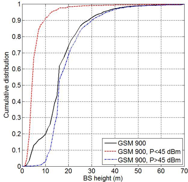
Figure 9. Distribution of MFCN base station antenna heights for a specific GSM-900 deployment.
