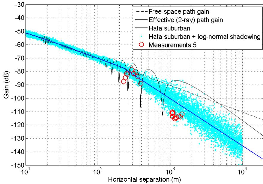
Figure 53. Comparison of field measurements with the propagation model used in this report. Base station antenna height of 15 m (Snowdome). Lobe at 0.3 – 0.4 km suggests constructive ground reflection. Measured path loss at larger separations are far greater than predicted by two-ray null pattern. This is possibly due to the low base station antenna height (below local tree line).
