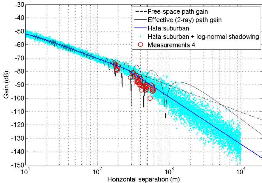
Figure 52. Comparison of field measurements with the propagation model used in this report.
