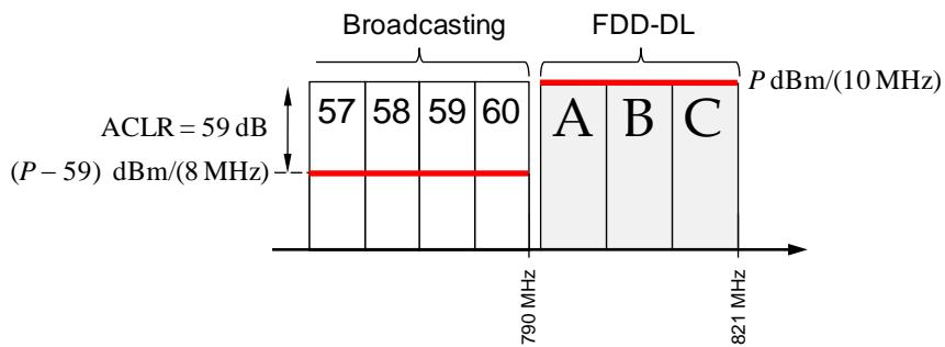
Figure 17. The EC Decision BEM for MFCN base stations, specified in relation to the 790 MHz frequency boundary. Filtering at the base station transmitters must result in a minimum ACLR of 59 dB.
