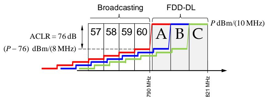
Figure 18. Assumed spectral leakage of the MFCN base stations. The emission masks are specified with reference to the carrier frequencies in blocks A, B, and C.
