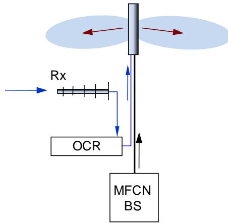
Figure 30. Antenna sharing between OCR and base station.
