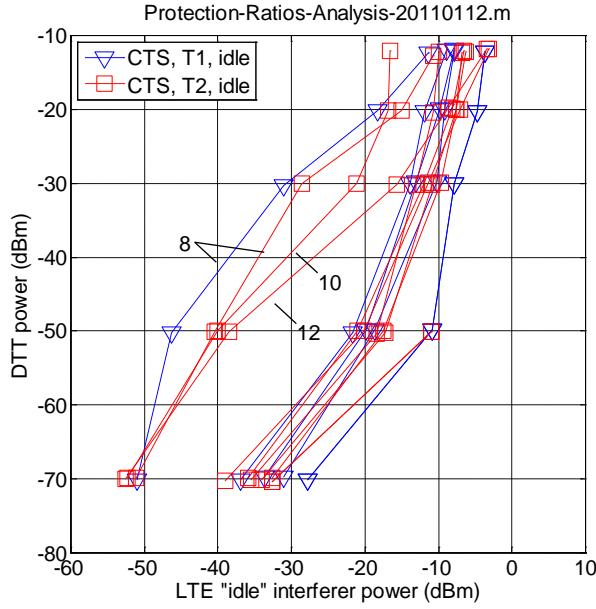
Figure 59. ERA raw protection ratio measurements (channel 60).
