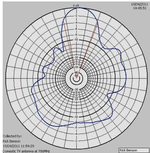
Figure 24. Angular discrimination gain of the tested domestic TV antenna.
