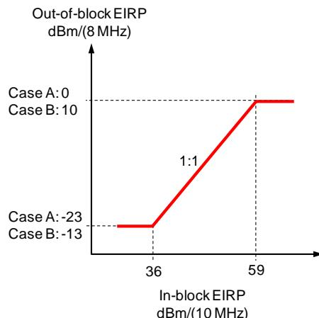
**Figure 4. Relationship between base station in-block and out-of-block EIRP limits.**
