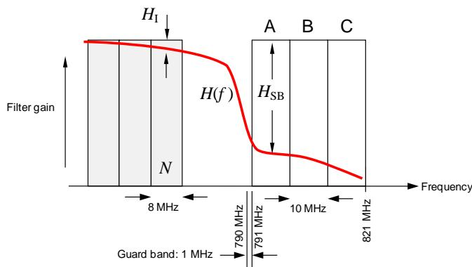
Figure 14. Typical frequency response of a type-N filter used for the protection of DTT channels  $N$  and below.
