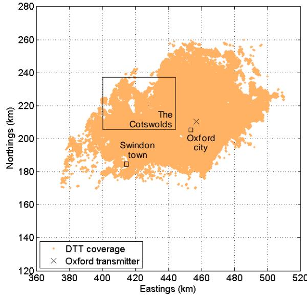
Figure 11. Coverage area of the Oxford transmitter. DTT coverage refers to pixels where the location probability is greater than 70%.
