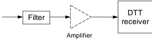
Figure 13. Filtering at the input to a DTT receiver.
