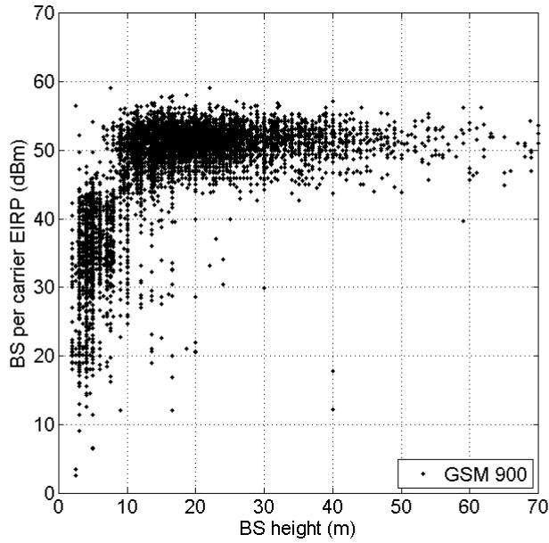
Figure 8. Correlation between GSM-900 base station EIRP(per carrier) and antenna height.
