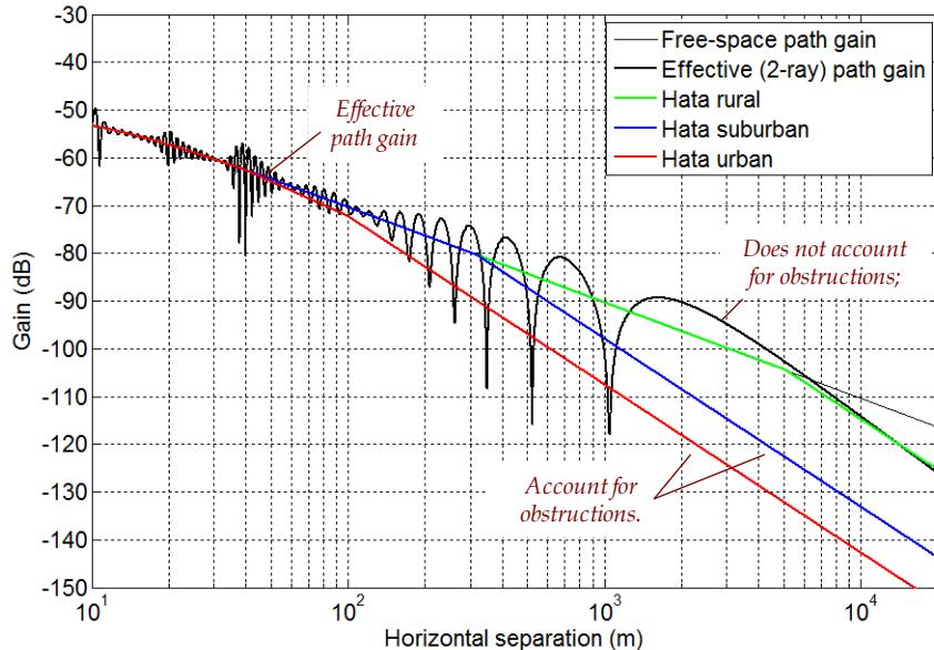
Figure 44. Comparison of effective (two-ray) path gain and extended-Hata models.
