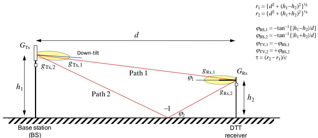
Figure 39. Two-ray propagation: geometry.
