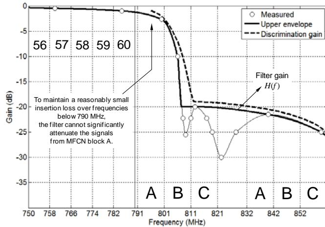
Figure 15. Frequency discrimination gain for a type-60 filter prototype by Technetix.
