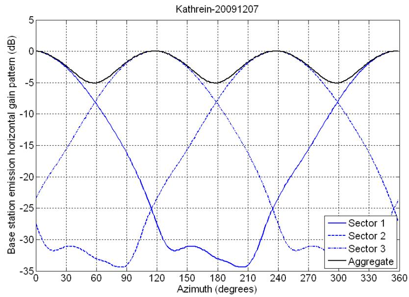
Figure 37. Kathrein antenna angular discrimination in azimuth.
