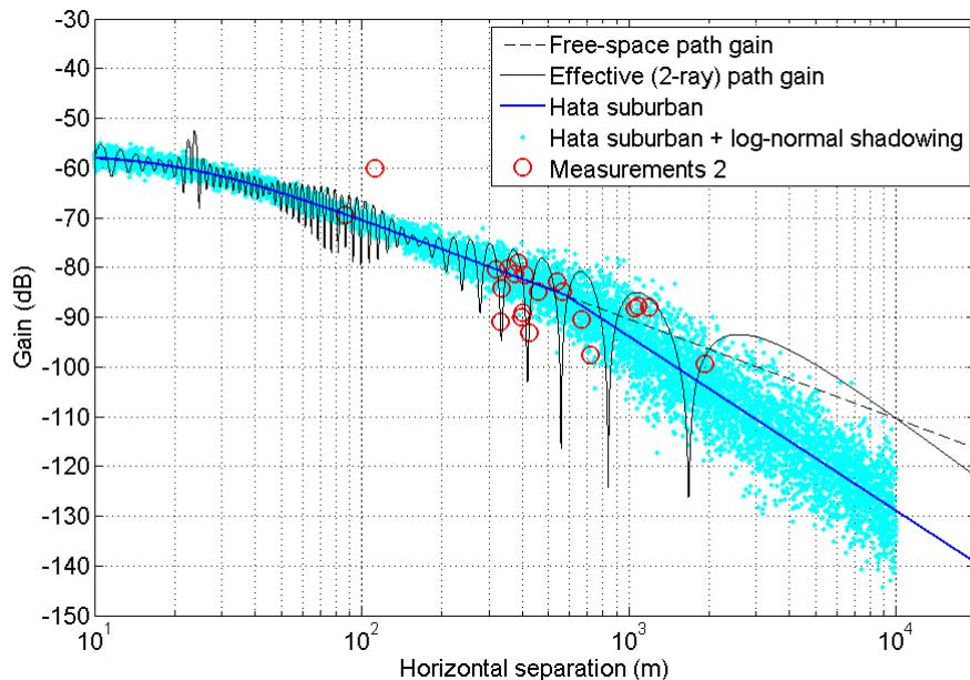
Figure 50. Comparison of field measurements with the propagation model used in this report.
