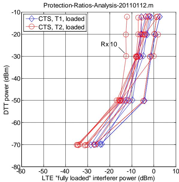
Figure 58. ERA raw protection ratio measurements (channel 60).
