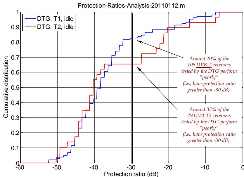
Figure 63. Cumulative distribution of DTG protection ratio measurements (channel 60).
