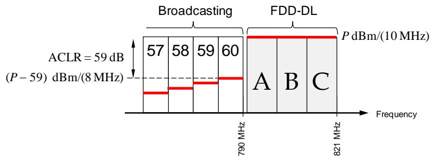
Figure 16. Assumed spectral leakage of the MFCN base stations.
