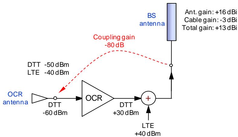
Figure 33. Physical arrangement and implications for coupling gain.
