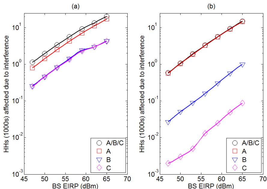
Figure 28. Variation of affected households in channel 60 as a function of base station EIRP for two cases: a) no filtering, b) filtering at the base station transmitters and DTT receivers.
