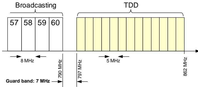
Figure 2. Frequency arrangement for TDD.
