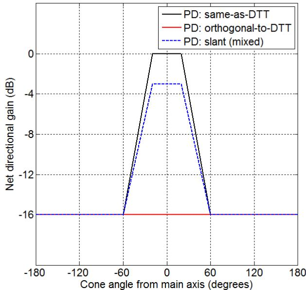
Figure 22. TV aerial net directional gain (combination of directional gain and polarisation discrimination) as a function of cone angle of arrival with respect to the aerial's main axis.
