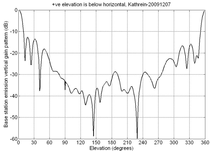
Figure 38. Kathrein antenna angular discrimination in elevation.
