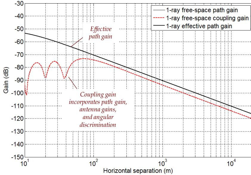
Figure 42. Effective path gain consistent with single-ray propagation.
