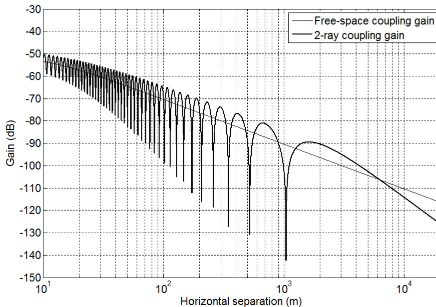
Figure 40. Free-space and two-ray coupling gains.
