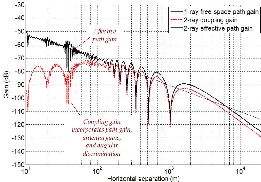
Figure 43. Two Effective path gain consistent with two-ray propagation.
