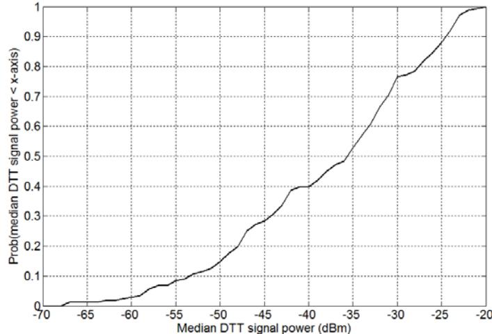
Figure 34. Distribution of DTT signal strength at the locations of an operator's GSM-900 base stations. Derived for the APSA coverage area of the Oxford transmitter, assuming a 9.15 dBi antenna gain at a height of 10 m.
