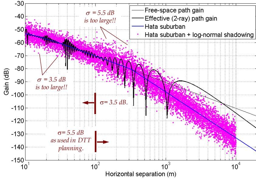
Figure 46. Comparison of effective two-ray path-gain and suburban-Hata with the SE42 log-normal standard deviation profile.
