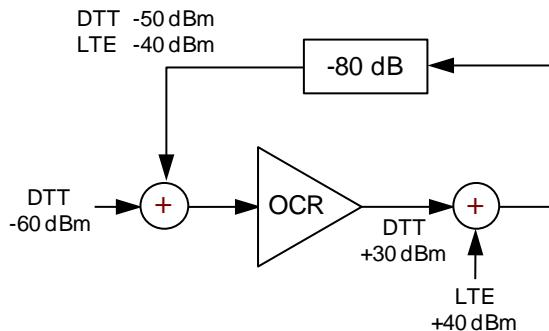
Figure 32. Bench test set-up.
