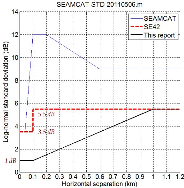
Figure 45. Standard deviation of log-normal shadowing.
