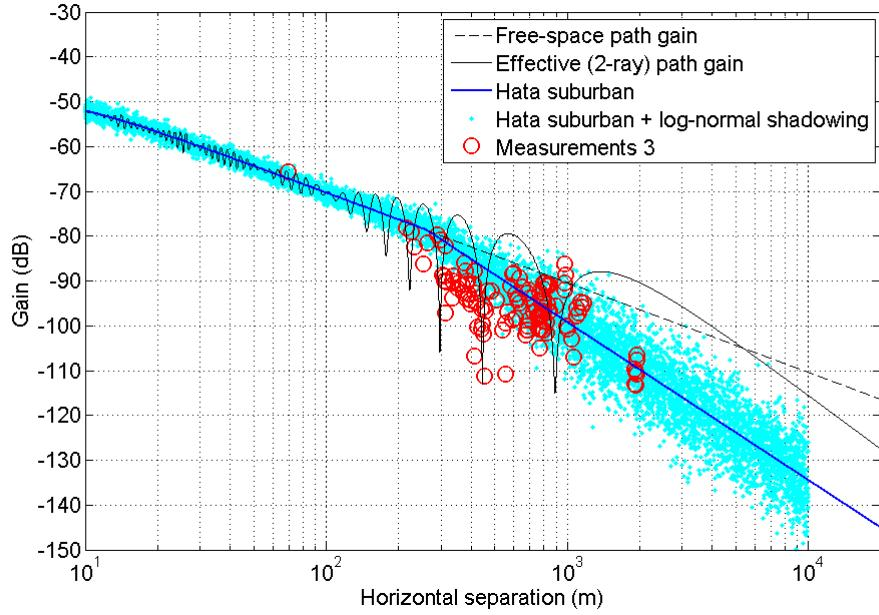
Figure 51. Comparison of field measurements with the propagation model used in this report.
