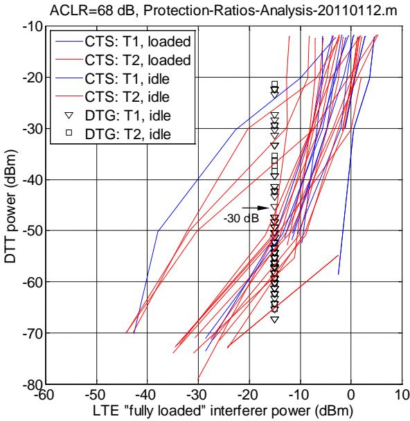
Figure 62. DTG and ERA post processed measurements (channel 60)
