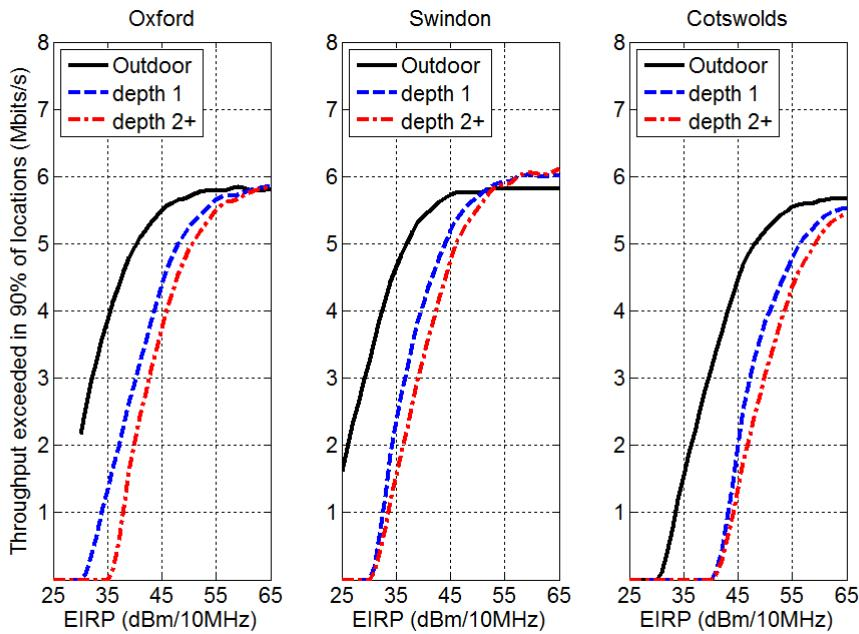
Figure 29. Variation of LTE downlink single-user throughput at cell-edge as a function of base station EIRP. MIMO: 2×2.
