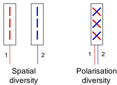
Figure 20. Spatial vs. polarisation diversity used to implement multi-antenna techniques at MFCN base stations.
