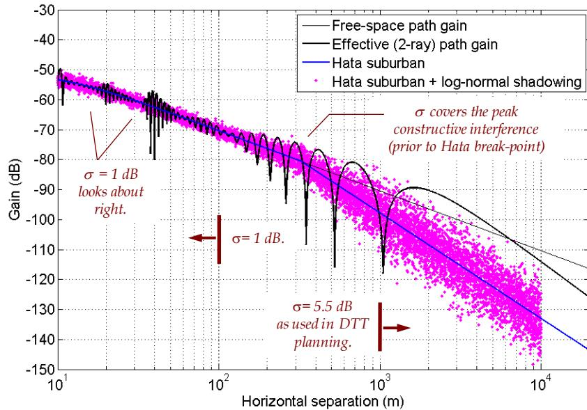
Figure 47. Comparison of effective two-ray path-gain and suburban-Hata with the revised log-normal standard deviation profile.
