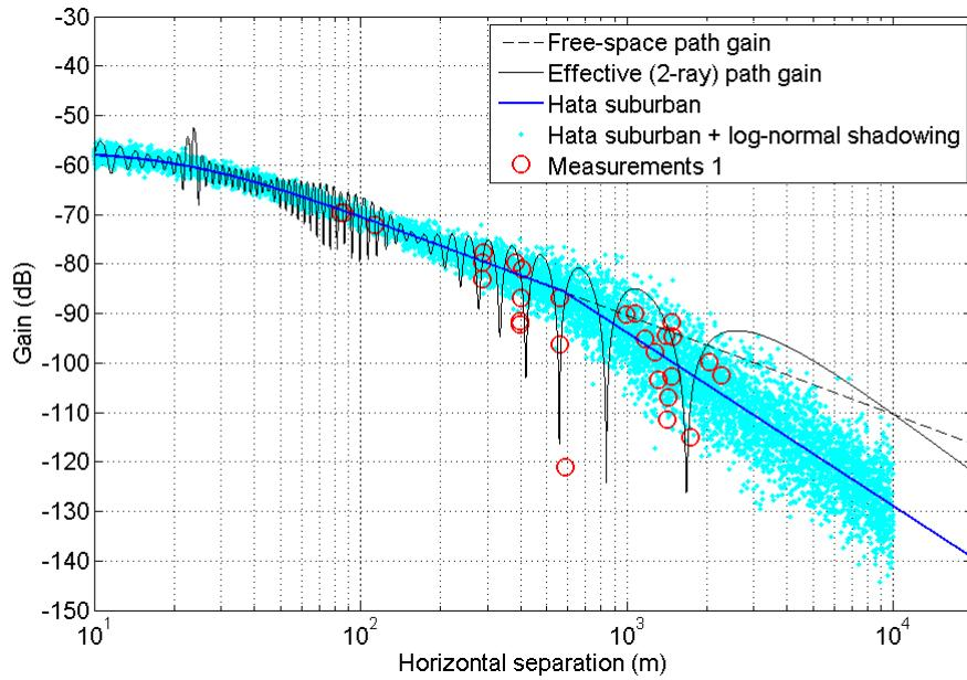
Figure 49. Comparison of field measurements with propagation model used in this report.
