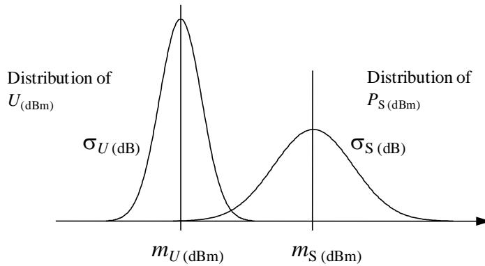
Figure 5. Distributions of wanted DTT power and DTT-to-DTT interference power in a pixel.
