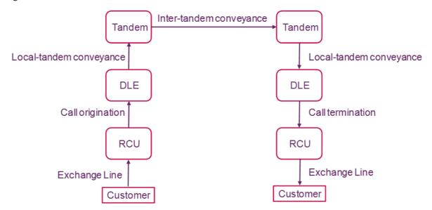
Figure 2.2: BT's voice network architecture
