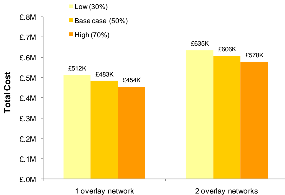
Figure 14: Total costs in suburban geotype at 31% penetration with alternative assumptions for final drop duct reuse
