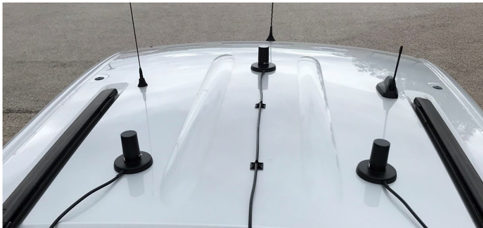
Figure 4: Top view of antennas mounted on a Renault Kangoo
