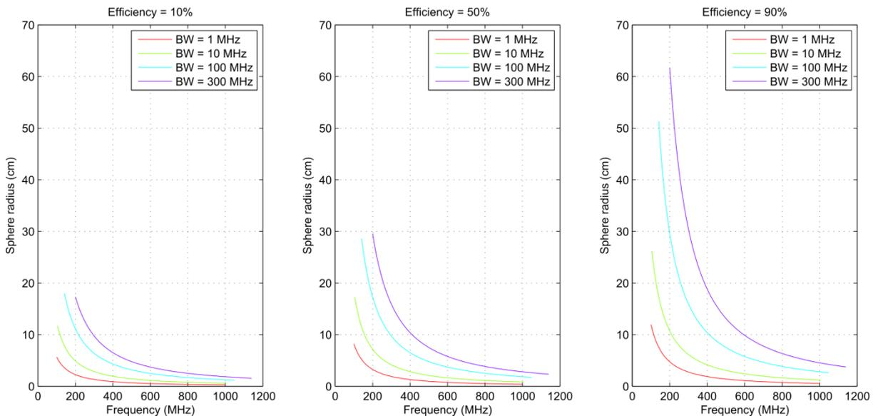
**Figure 1: Antenna size versus frequency for different efficiencies**
