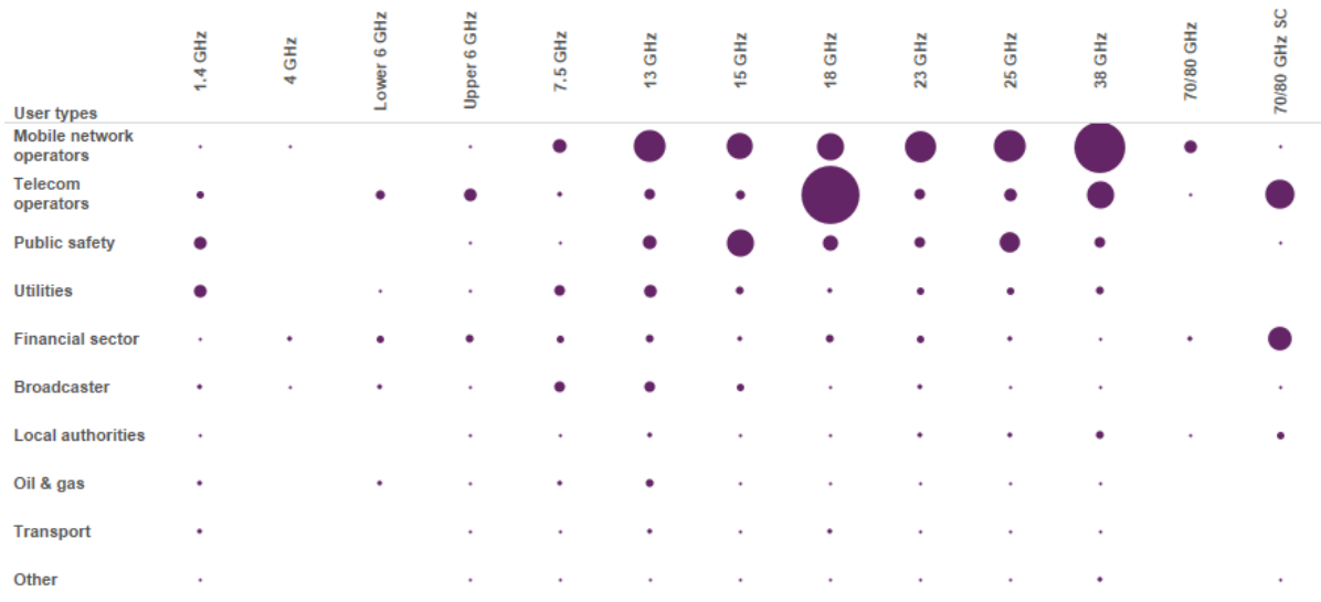
Figure 1: Initial categorisation of Fixed Service spectrum managed by Ofcom with usage shown by user types – the size of the circle is relative to the number of fixed wireless links licensed in the UK
