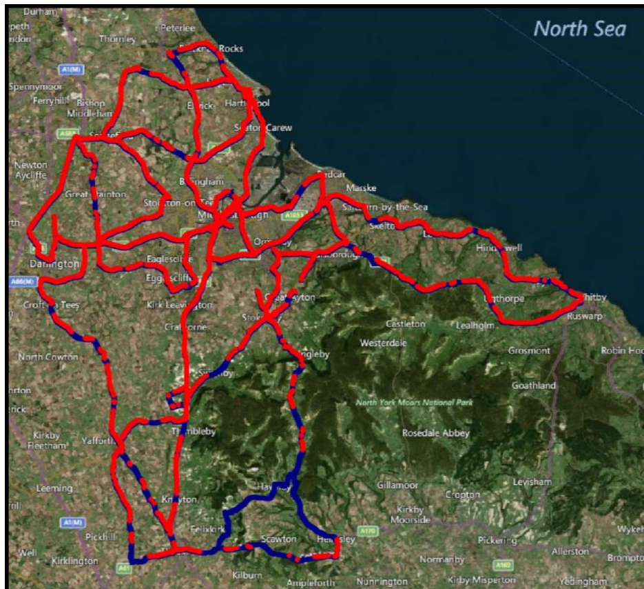
Figure 1: Areas where 4G coverage at a signal strength of at least -95 dBm is available (red) and is not available (blue), for at least one of the operators, for an area of Northern England.
