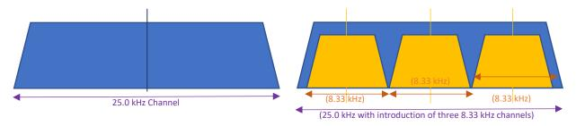
As an example, if we take the original transmit frequency 118.025MHz for a 25kHz channel we can split this into three new 8.33 kHz channels with transmit frequencies:
