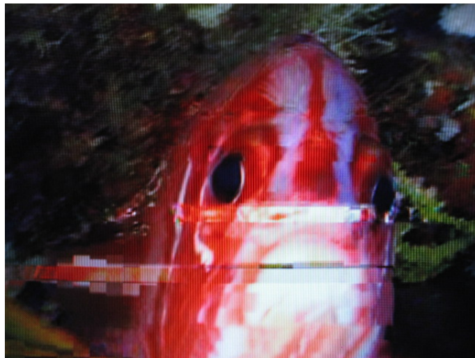
Figure 5: Picture showing typical interference observed on the LCD display from 3G and WiMAX signals
