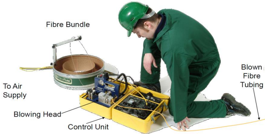
Figure 6.1: Equipment for blowing fibre installation [Source: Emtelle, 2012]
