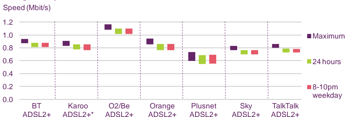
Figure 2.10 Maximum, average and peak-time upload speeds for ADSL2+ ISP packages: May 2012
