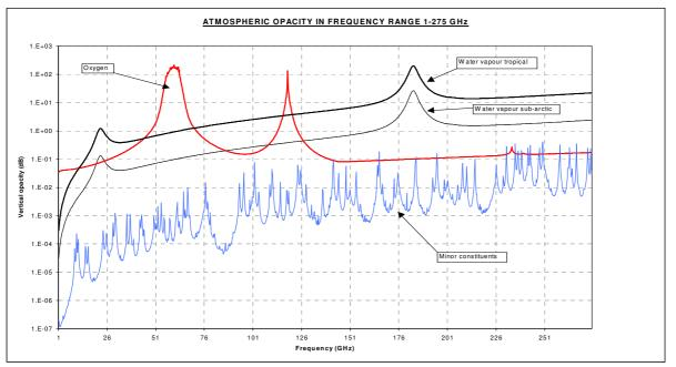
the many minor resonances and atmospheric windows where there is relatively low absorption, for example around 35 GHz, 90 GHz and 135 GHz are also important.
