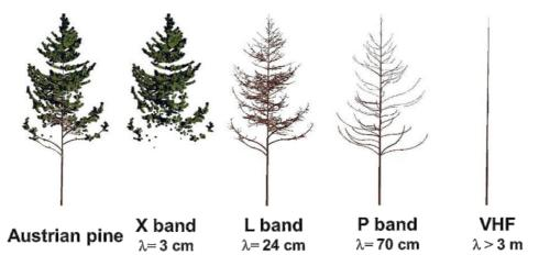
Figure 6 – Radar returns from vegetation at various wavelengths
