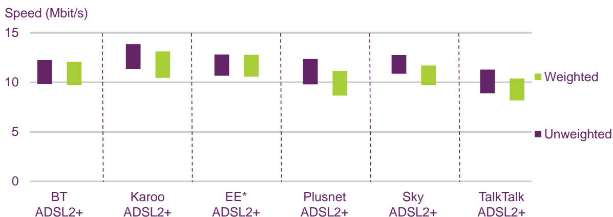
Figure 6.6 Maximum download speeds for ADSL2+ ISP packages, weighted and unweighted figures: May 2014
