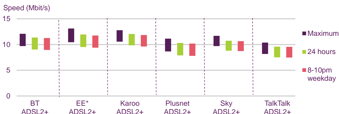
Figure 2.1 Maximum, average and peak-time download speeds for ADSL2+ ISP packages: May 2014
