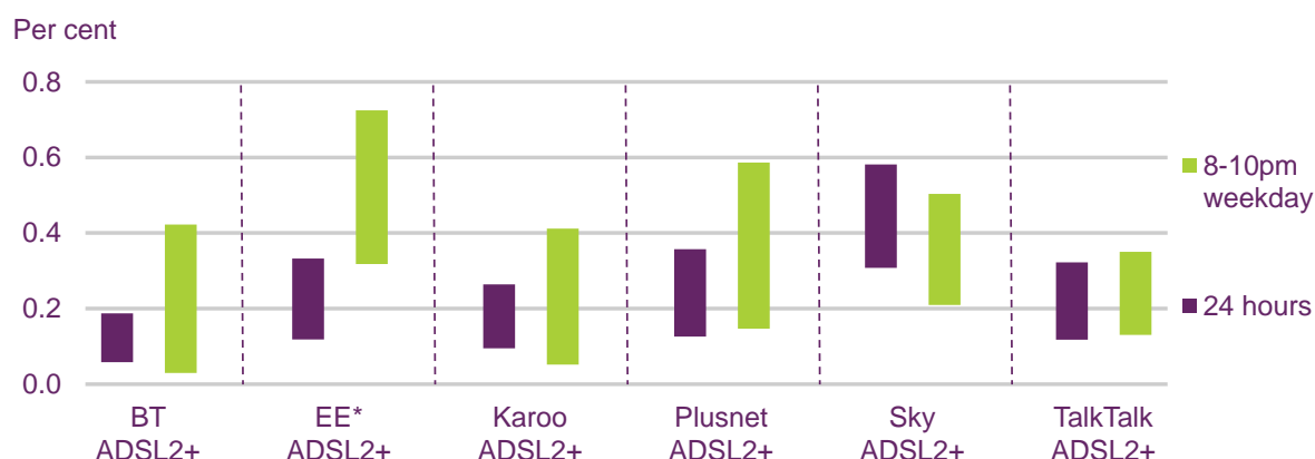
Figure 3.10 Average and peak-time packet loss for ADSL2+ ISP packages: May 2014
