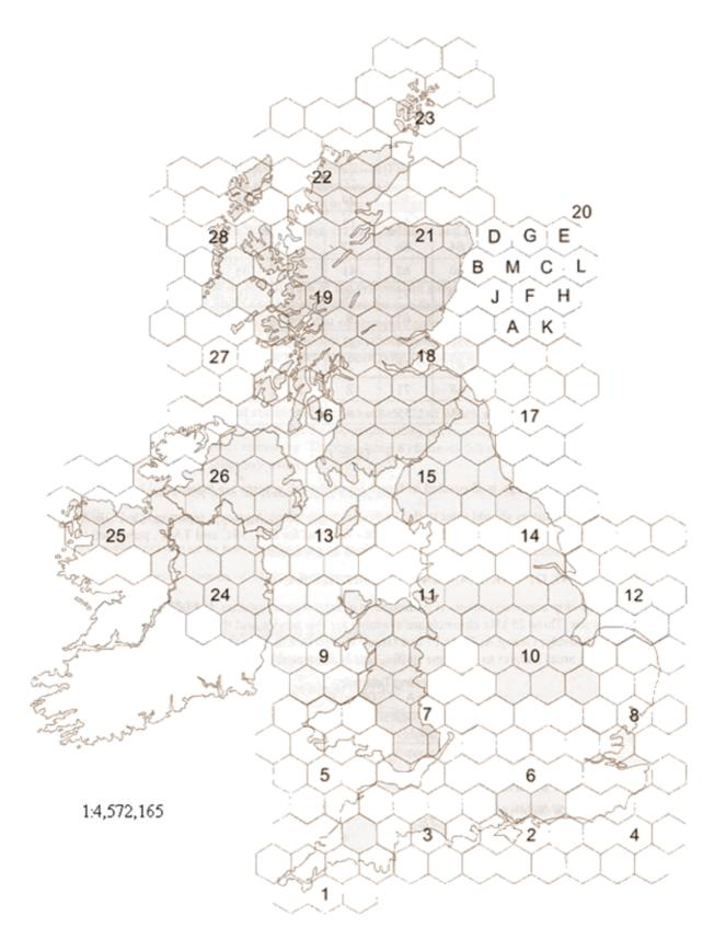
Figure 1: UK Cellular Plan for Scanning Telemetry and Telecontrol Services for the Utilities.
