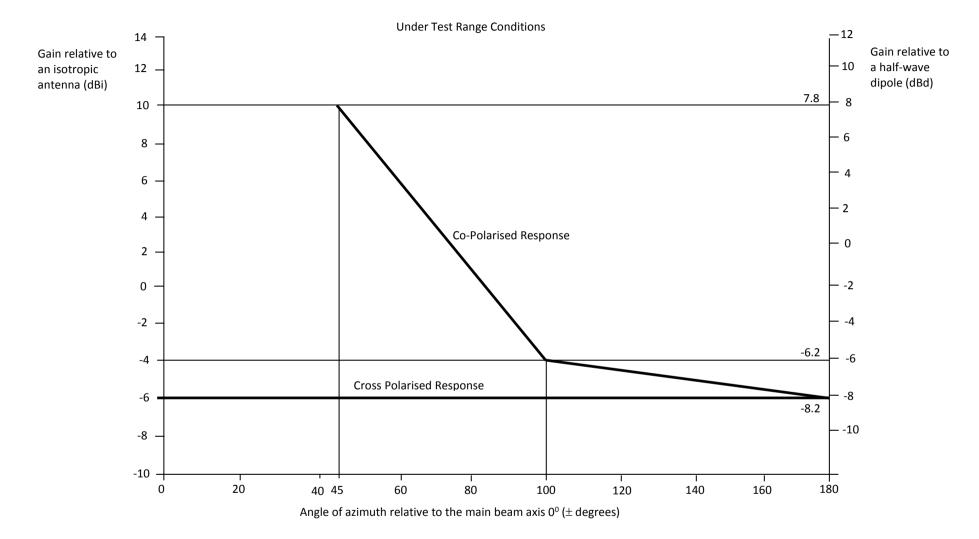
Figure 2: Sector Antenna Radiation Pattern Envelope for Base Stations
