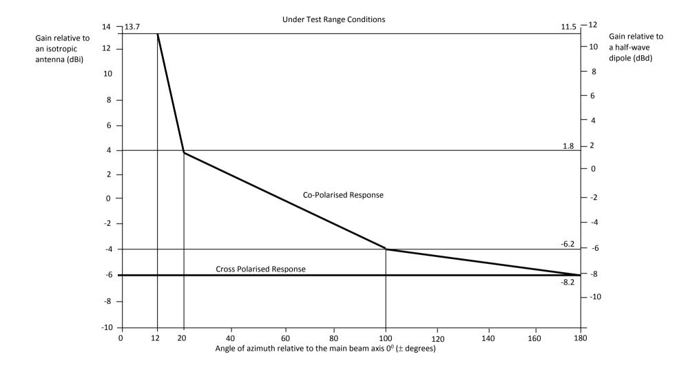
Figure 3: Antenna Radiation Pattern Envelope for Outstations – High Performance Antenna
