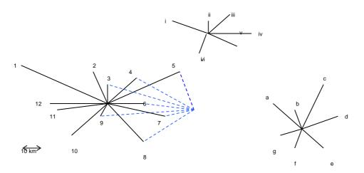
Figure 10: The same scanner-outstation family employing sectorisation and secondary receiver techniques
