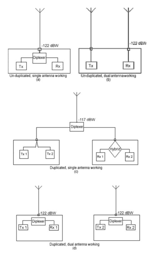
Note: The receiver levels in the diagrams above are for Outstation Class 1, for other Outstation classes these values will be different, refer to table 5 for more details.
