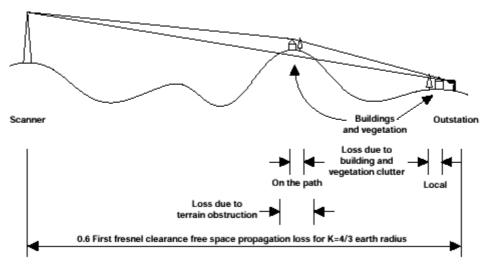
Figure 5: Losses along a path
