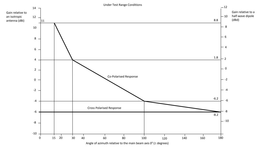
Figure 4: Antenna Radiation Pattern Envelope for Outstations – standard antenna
