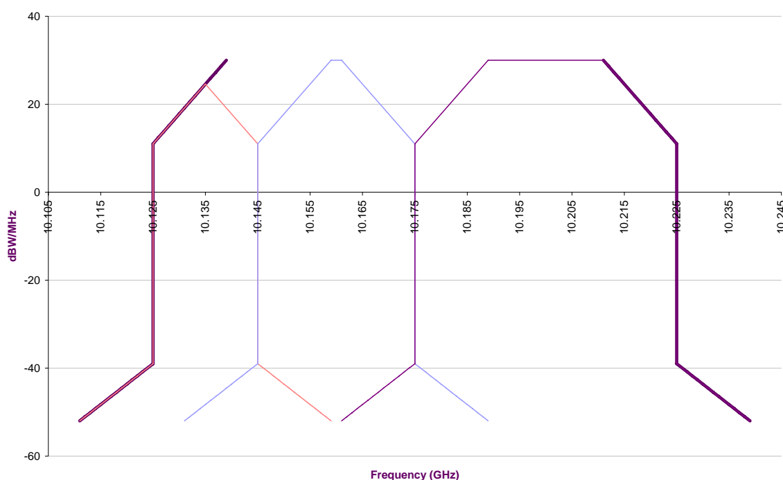
Figure 2. Illustration of the application of the spectrum mask to blocks of differing size
