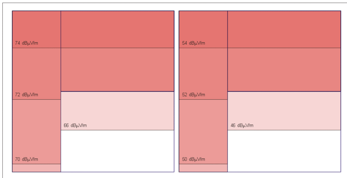
Figure 15 - Levels permitted at 220 MHz by EN 50121-2, rails 10m from the office. Left: peak levels (derived directly from the standard); right: estimate of quasi-peak levels (to calculate interference to radio service).
