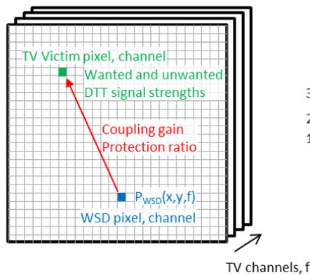
C) Output is max allowable WSD power for each channel, for the chosen pixel
