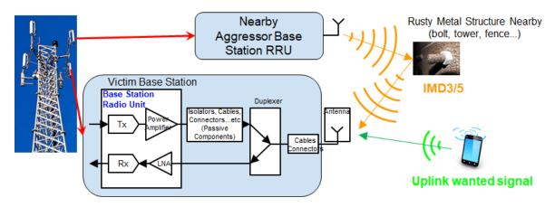
Base station receiver being impacted by external components such as rusty components which act as non linear transmitters and create inter-modulation products
