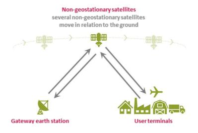
2.10 Satellite broadband services tend to operate in a small number of radio frequency bands (these are known as C band, Ku band, and Ka band<sup>2</sup>). Within these bands, different services use the same radio frequencies. The signals are coordinated – under international rules laid down in International Telecommunication Union (ITU) Radio Regulations – whenever
