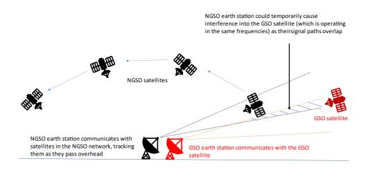
Figure 5: Potential for NGSO services to cause interference into GSO earth stations (space to Earth) as the NGSO satellites pass in front of the GSO arc
