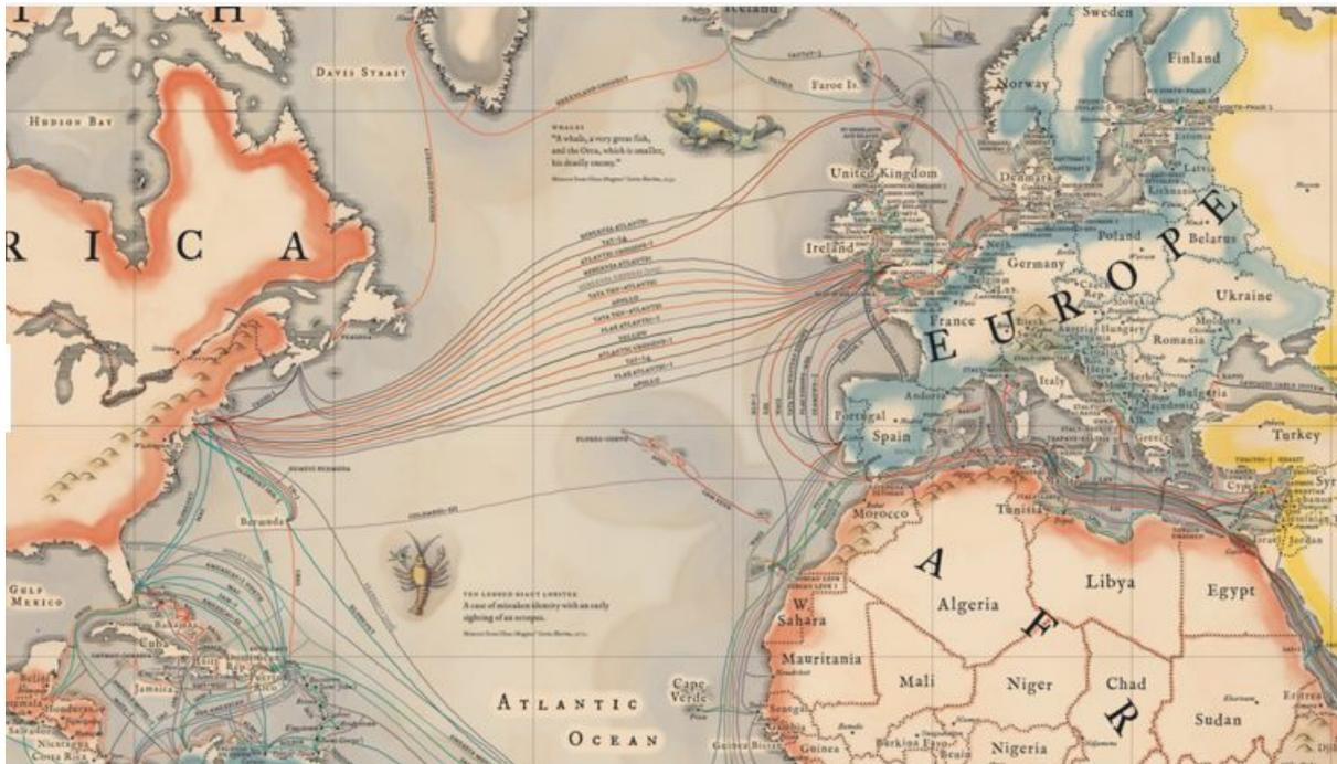
*Trade Routes of the 21<sup>st</sup> Century: Current Undersea Fibre Communications Cables which carry all of the worlds Internet traffic. (NB. Today, only in exceptional cases does internet data traffic travel via satellite because signal latency via satellite slows internet traffic more than is acceptable)*
