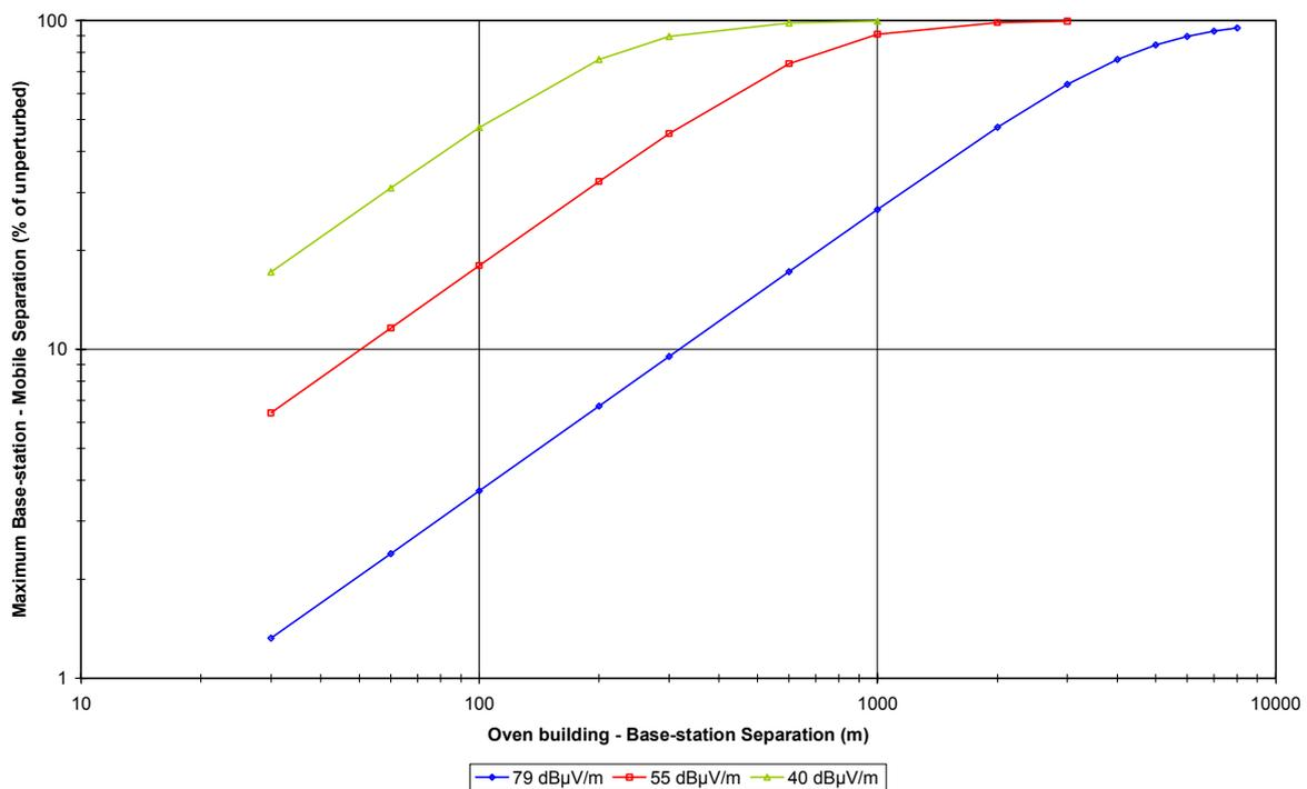
**Figure 2 - Maximum mobile phone – base-station separation (%) as a function of oven-building – base-station separation.**
