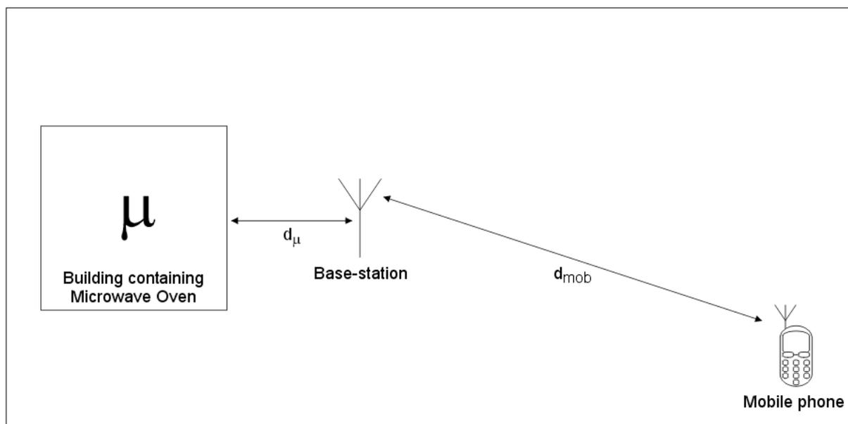
**Figure 1 - The scenario presents an oven  $\mu$  interfering with a base-station  $d_{\mu}$  distant such that a mobile phone cannot transmit to it beyond a maximum distance  $d_{mob}$ .**
