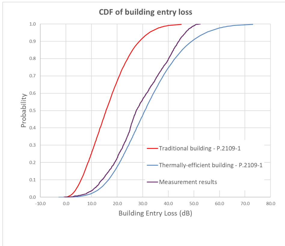
Figure 12 Probability of building entry loss derived from ground floor measurements in our London office
