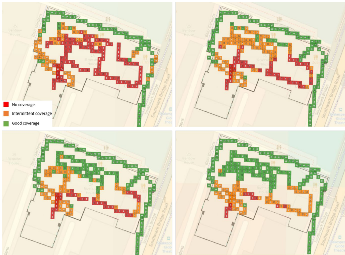
Figure 2 Mobile signal strength measurements in the 3.4 GHz band inside and outside Ofcom Riverside House office for the four MNOs
