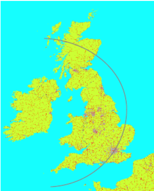
Figure 3: The predicted worst-case interference boundary from the Republic of Ireland's digital broadcasts within DVB-T channel CH8.
