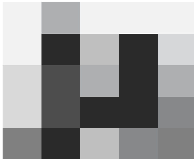
Figure 5. Each sub-image is labelled 1 or 0 based on whether its colour is brighter or darker than the average of all sub-images.
