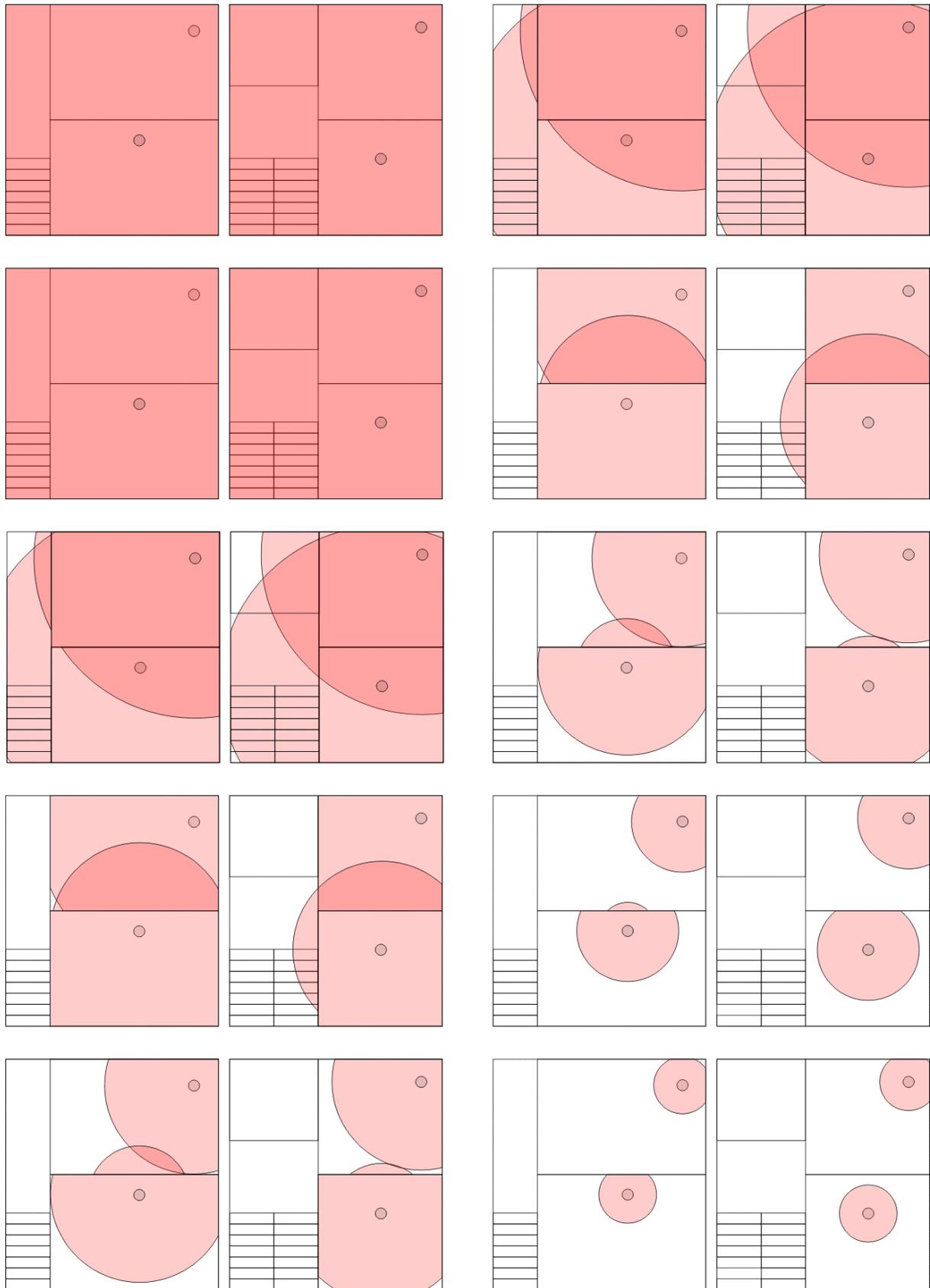
**Figure 3: Region of disturbance for GSM900 signal strengths of 47.3, 52.3, 57.3, 62.3 and 67.3 dB $\mu$ V/m (top to bottom), left hand side drawings show devices emitting 10 dB above CISPR 22 limits, right hand side drawings show devices just meeting CISPR 22 limits.**
