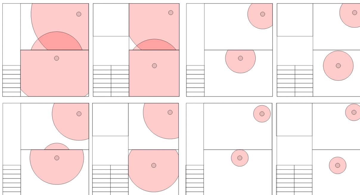
**Figure 2 - Region of disturbance for DVB-T signal strengths of 76 (top) and 81 dB $\mu$ V/m (bottom), left hand side drawings show devices emitting 10 dB above CISPR 22 limits, right hand side drawings show devices just meeting CISPR 22 limits.**
