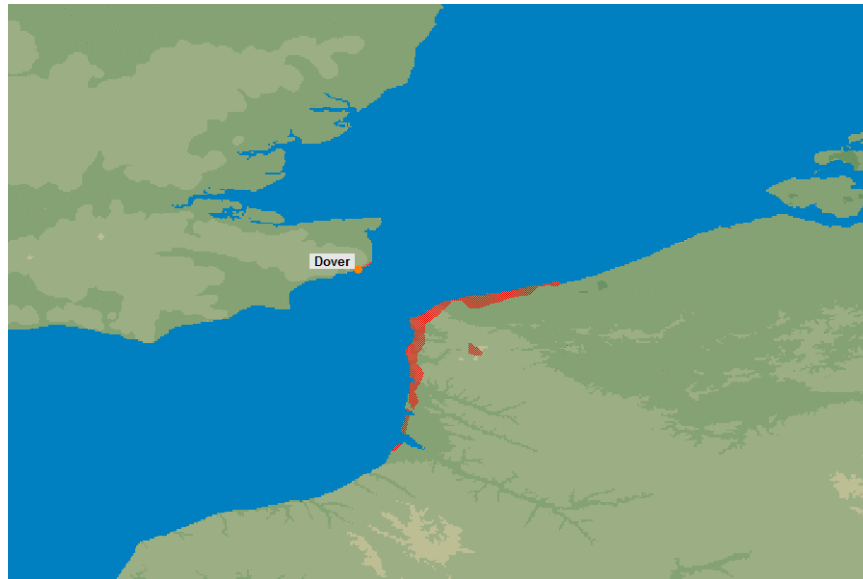
Figure 31: Interference Area for UK Mobile Transmitter at Whitfield (Threshold: 20 dB \mu V/m in 25 kHz at 10 m for 10% of time, TX EIRP towards the Continent: 30 dBm / 25 kHz, TX Height: 1.5 m)
