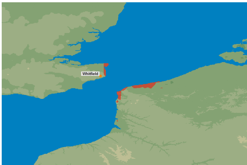
Figure 31: Interference Area for UK Mobile Transmitter at Whitfield (Threshold: 20 dB \mu V/m in 25 kHz at 10 m for 10% of time, TX EIRP towards the Continent: 30 dBm / 25 kHz, TX Height: 1.5 m)
