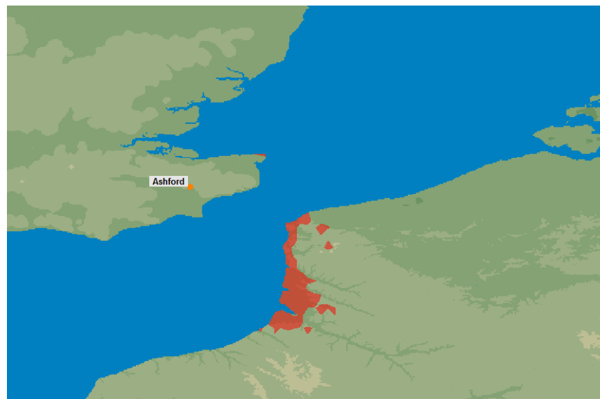
Figure 29: Interference Area for UK Transmitter at Ashford (Threshold: 20 dB \mu V/m in 25 kHz at 10 m for 10% of time, TX EIRP towards the Continent: 53 dBm / 100 kHz, TX Height: 30 m)
