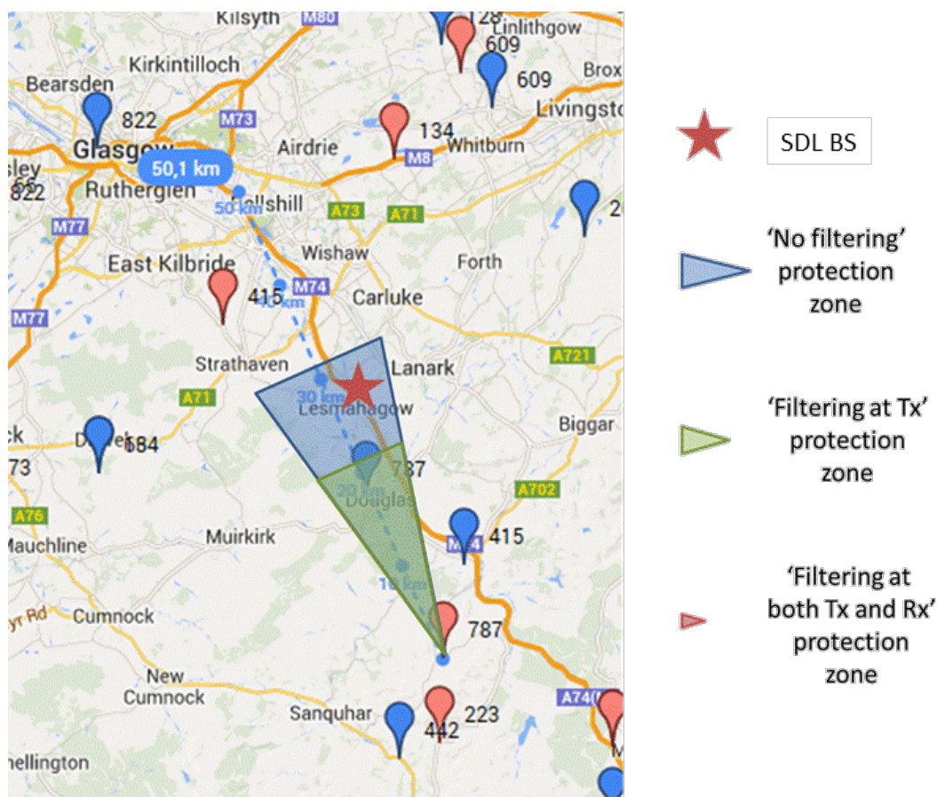
Figure 107: Impact of filtering on the protection zone
