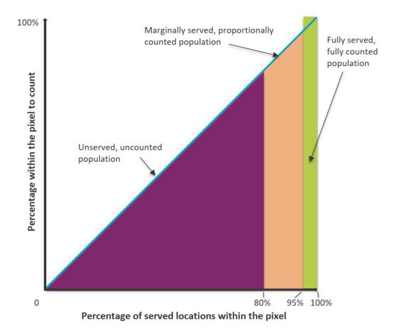
Figure 3: Diagrammatic representation of the proportional counting thresholds
