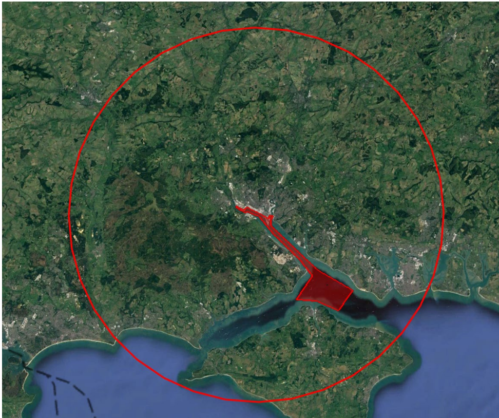
Figure 8: Port of Southampton example - PFD limited zone (inner) and coordination zone (outer)
