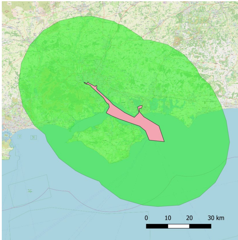
Figure 5.10: Illustration of a coordination zone defined as a polygon around the Southampton and the Solent PFD limited zone, for Phase 1 PFD limits and 'large cell' IMT deployments.
