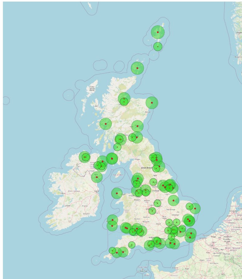
Figure 3.2: Locations of proposed Phase 1 PFD limited and coordination zones around major ports and international airports 13
