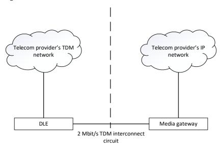
Figure 7.3: TDM interconnection between a TDM network and an IP network
