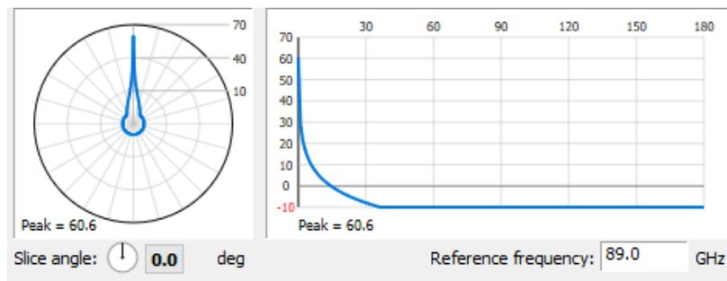
The antenna pattern envelope of the above figure for small off-axis angles is shown below. Implementation of S.580 antenna pattern envelope in Visualyse is slightly more conservative than the pattern envelope described in Section 1.1, which is based on combination of S.580 and Radio Regulation Appendix 7.
