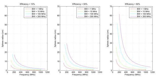
Figure 1: Antenna size versus frequency for different efficiencies
