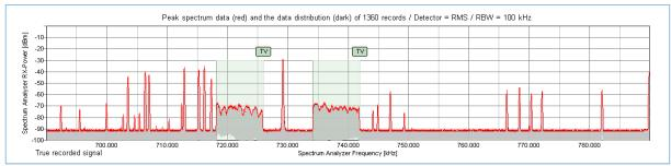
27 wireless microphones, IEM and audio links were coordinated in the band 690 to 790 MHz. The scanner has recorded approximately 26 carriers in the band 690 to 790 MHz.
