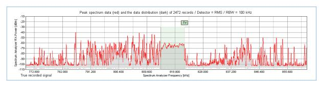
The licence exempt "microphone bands" 790 to 814 and 838 to 862 MHz are in heavy in-use. The scanner has recorded 113 carriercarriers within 3 days.
