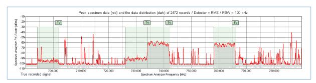
The scanner has recorded approximately 44 carrier in the band 690 to 790 MHz.
