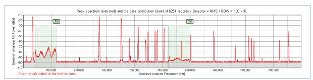
67 wireless microphones, IEM and audio links were coordinated in the band 690 to 790 MHz. The scanner has recorded approximately 25 carriers in the band 690 to 790 MHz.
