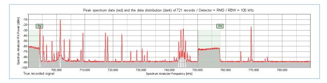
65 wireless microphones, IEM and audio links were coordinated in the band 690 to 790 MHz. The scanner has recorded approximately 28 carriers in the band 690 to 790 MHz.
