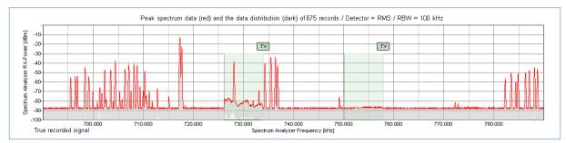
73 wireless microphones, IEM and audio links were coordinated in the band 690 to 790 MHz. The scanner has recorded approximately 39 carriers in the band 690 to 790 MHz.
