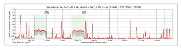
69 wireless microphones and IEM were coordinated in the band 690 to 790 MHz. The scanner has recorded approximately 30 carriers in the band 690 to 790 MHz.
