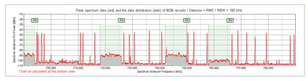
56 wireless microphones, IEM and audio links were coordinated in the band 690 to 790 MHz. The scanner has recorded approximately 36 carriers in the band 690 to 790 MHz.
