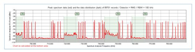
In the neighbourhood exhibition centre was taking part the trade fair "Interpack", at the same time Simultaneously with the Eurovision event "Interpack" was taking place in an adjacent Hall. - 56 wireless microphones, IEM and audio links were coordinated in the band 690 to 790 MHz. The scanner has recorded approximately 50 carriers in the band 690 to 790 MHz. Get dDetailed information in a detailed DKE report 15.
