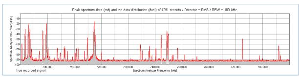
38 wireless microphones, IEM and audio links were coordinated in the band 690 to 790 MHz. The scanner has recorded approximately 39 carriers in the band 690 to 790 MHz.
