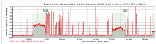
198 wireless microphones, IEM and audio links were coordinated in the band 470 to 862 MHz. Since no detailed data were available 147 wireless microphones and IEM were calculated the band 690 to 790 MHz.
