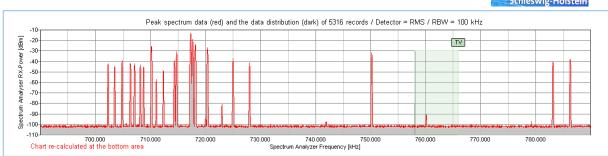
44 wireless microphones, IEM and audio links were coordinated in the band 690 to 790 MHz. The scanner has recorded approximately 29 carriers in the band 690 to 790 MHz.
