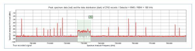
65 wireless microphones, IEM and audio links were coordinated in the band 690 to 790 MHz. The scanner has recorded approximately 18 carriers in the band 690 to 790 MHz.
