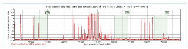
127 wireless microphones, IEM and audio links were coordinated in the band 690 to 790 MHz. The scanner has recorded approximately 37 carriers in the band 690 to 790 MHz.
