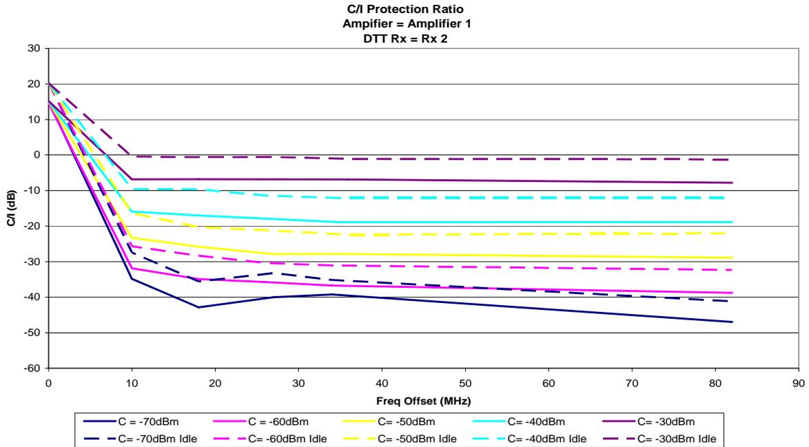
Figure 46: Amplifier 1 (masthead) with Rx2, without the use of filtering
