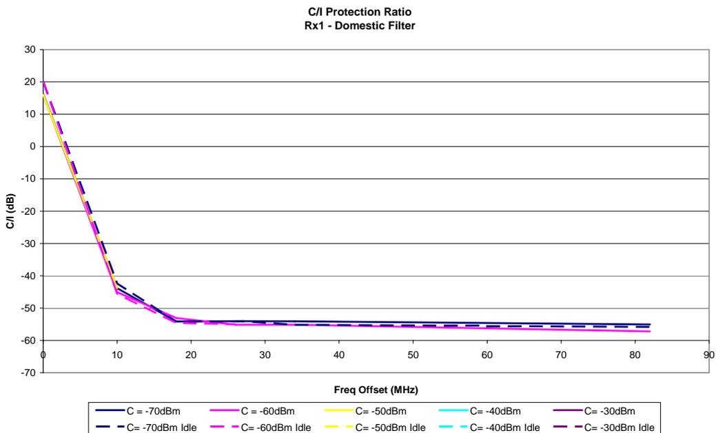
Figure 31: DTT Receiver 1 performance with filtering
