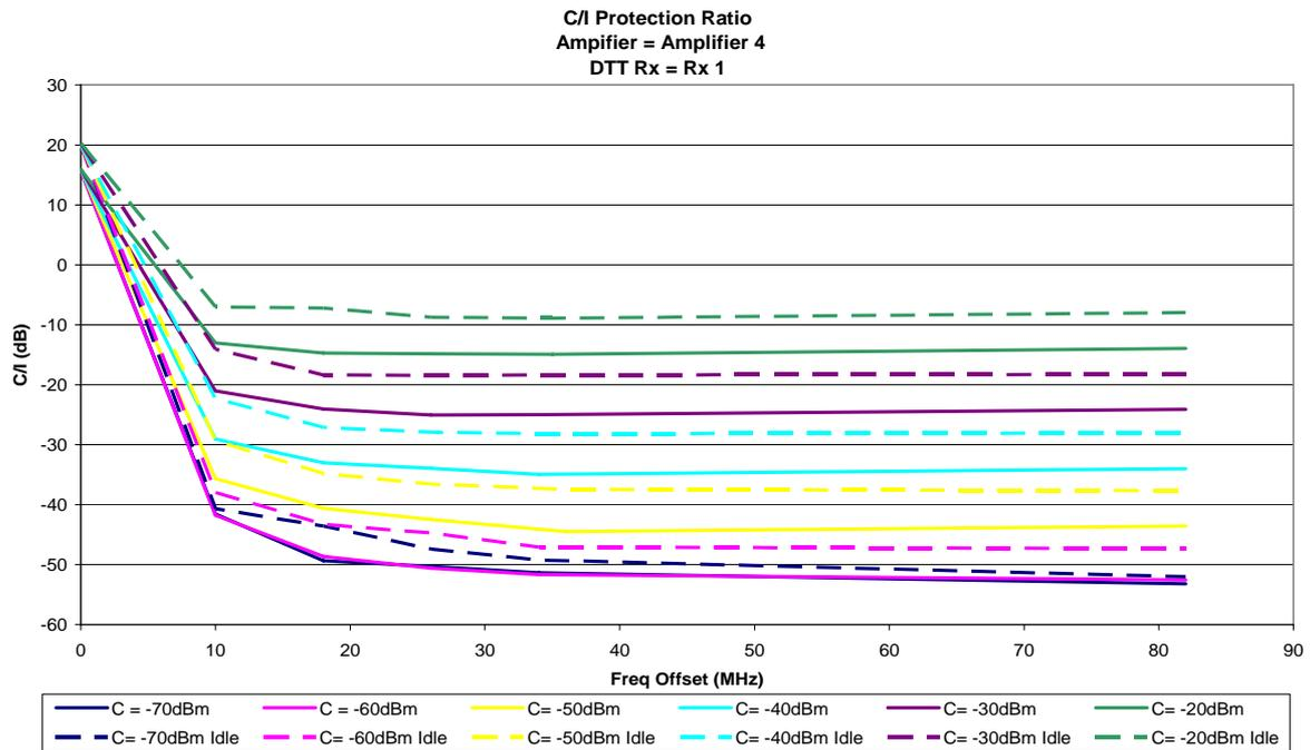
**Figure 40: Amplifier 4 (indoor) with Rx1, without the use of filtering**
