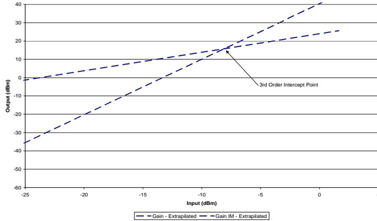
Figure 24: Amplifier 1 (masthead) 3<sup>rd</sup> order intercept point
