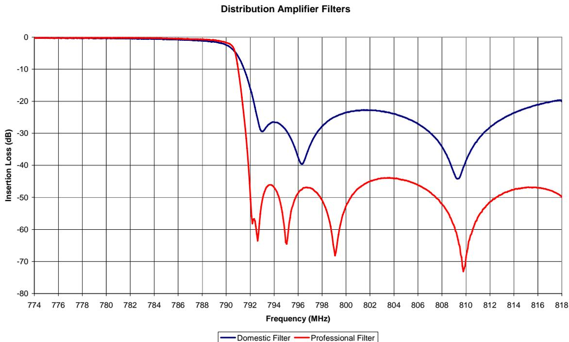
**Figure 3: Filter rejection in Block A (791 – 801 MHz)**
