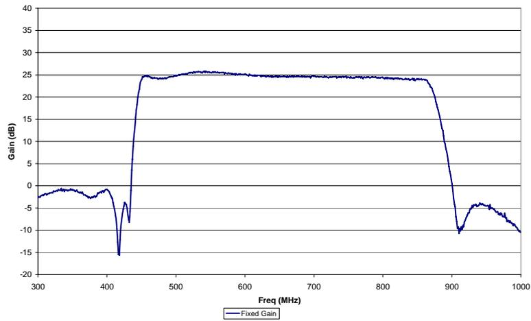
Figure 12: Amplifier 1 (masthead) gain response
