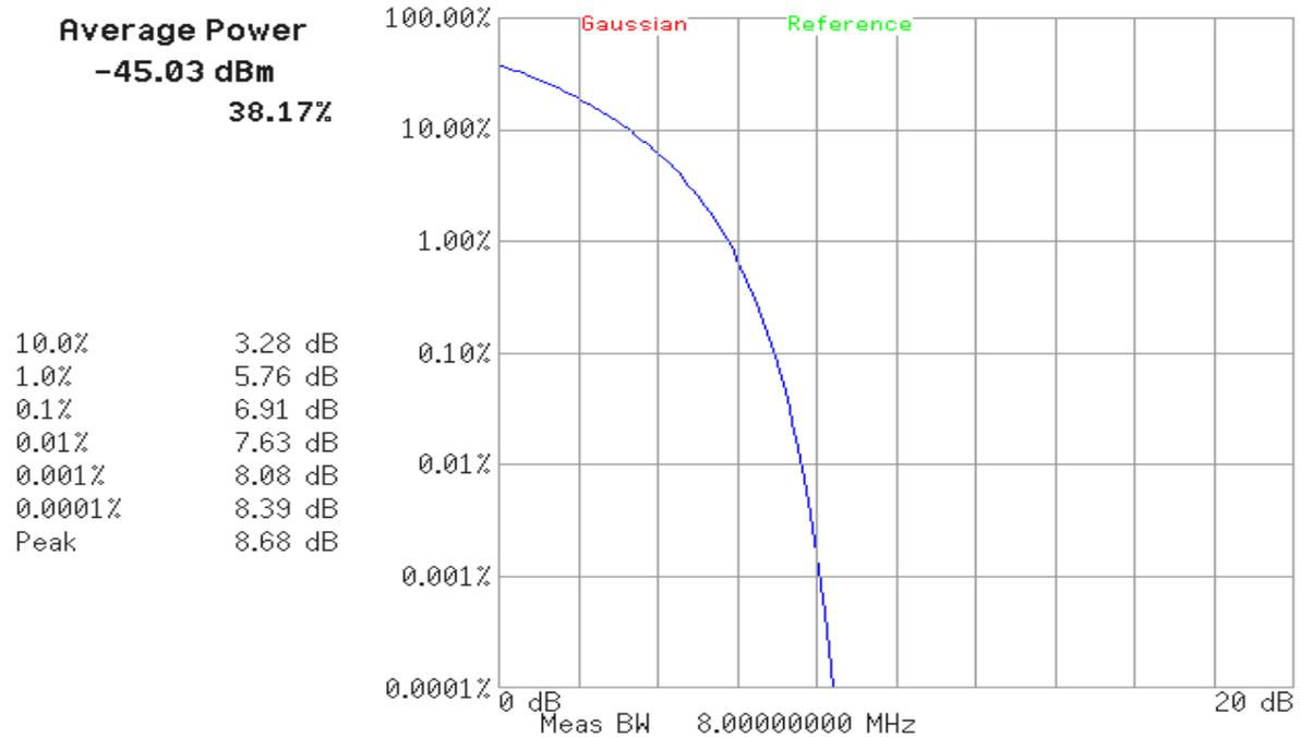
Figure 58: CCDF Measurement of LTE 100% (fully loaded) Signal
