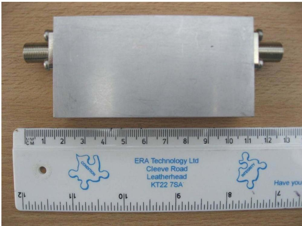
Figure 2: Prototype domestic filter for use with indoor amplifiers
