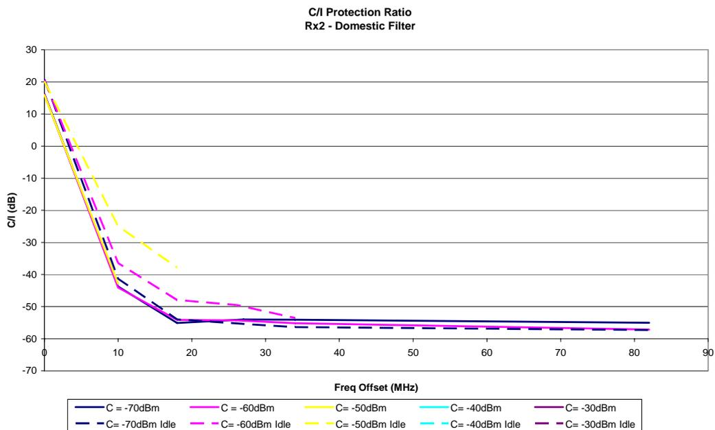
**Figure 33: DTT Receiver 2 performance with filtering**
