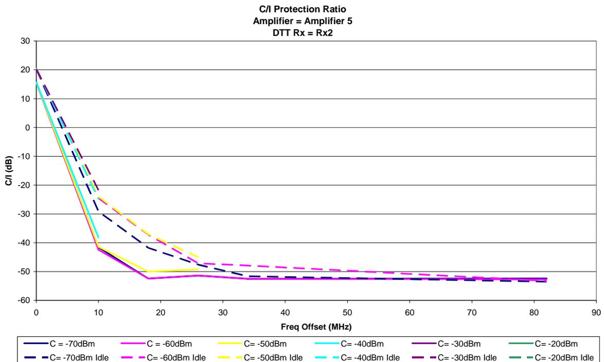
Figure 55: Amplifier 5 (indoor) with Rx2, with filtering
