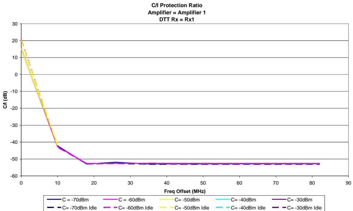
Figure 35: Amplifier 1 (masthead) with Rx1, with filtering
