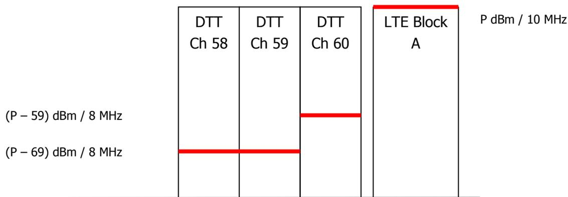
**Figure 11: Graphical representation of LTE emissions**
