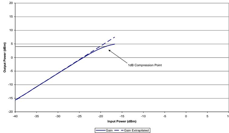
Figure 18: Amplifier 1 (masthead) 1 dB compression point
