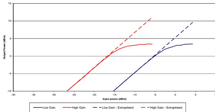
Figure 22: Amplifier 5 (indoor) 1 dB compression point
