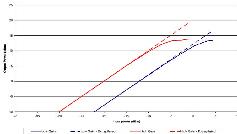
Figure 23: Amplifier 6 (indoor) 1 dB compression point
