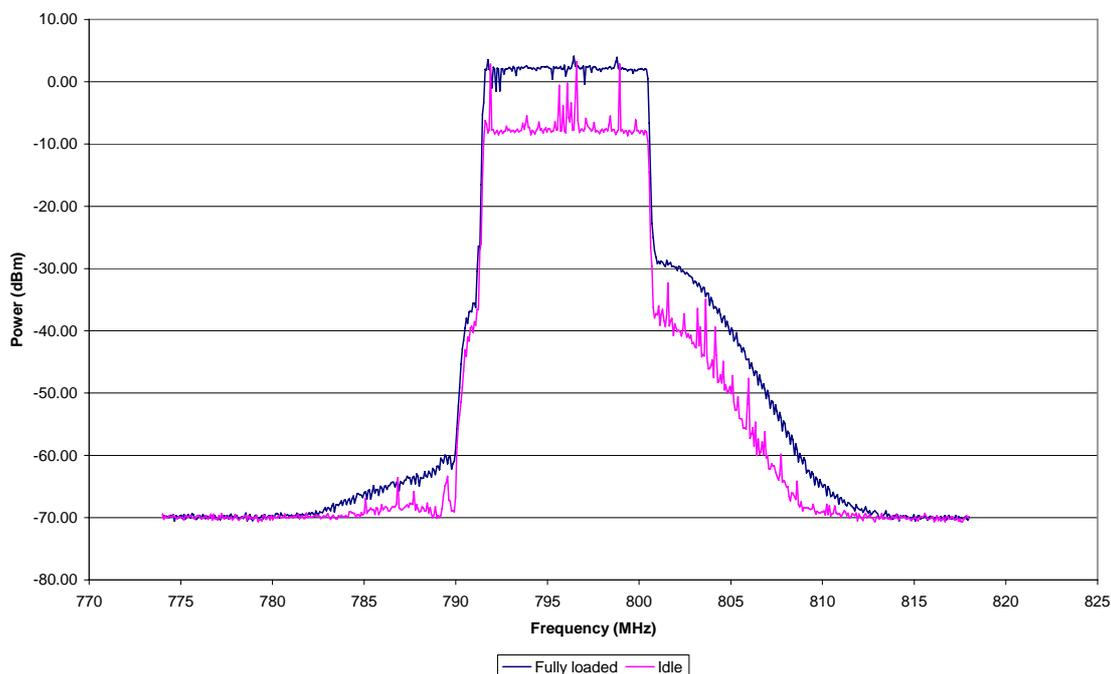
**Figure 9: Comparison of fully loaded and idle base station emissions**
