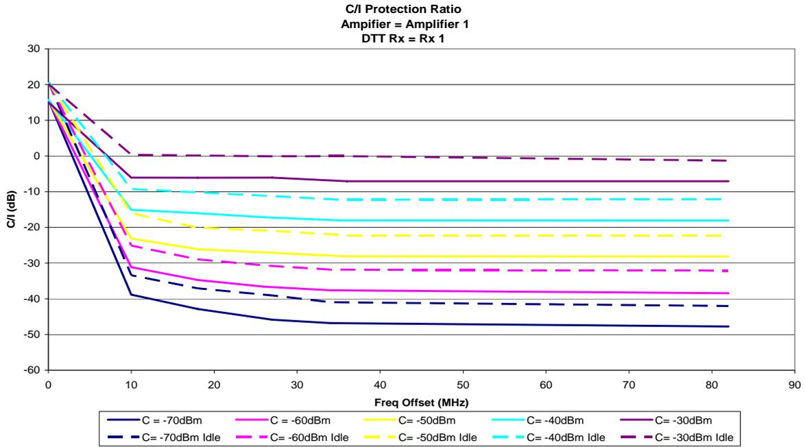
Figure 34: Amplifier 1 (masthead) with Rx1, without the use of filtering
