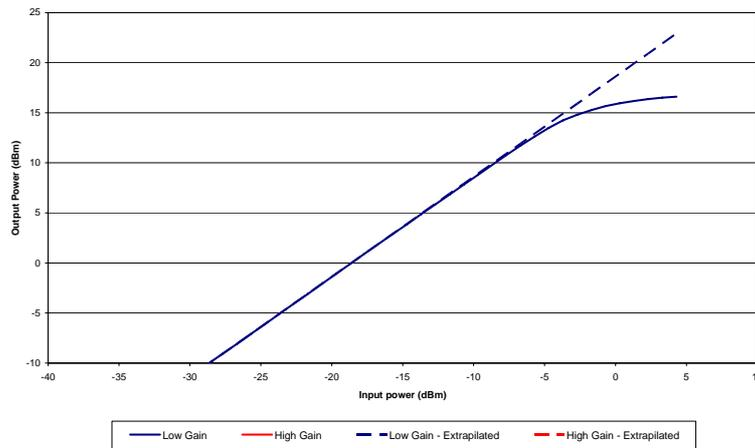
Figure 21: Amplifier 4 (indoor) 1 dB compression point
