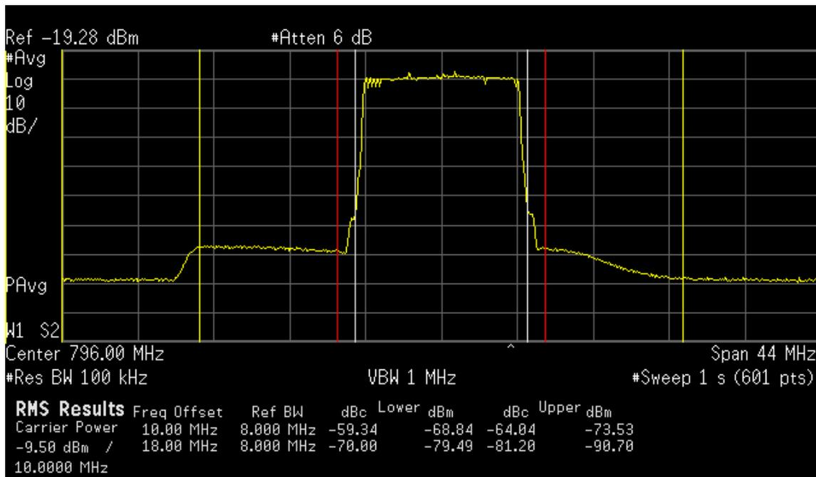
Figure 7: LTE base station emission under fully loaded traffic conditions
