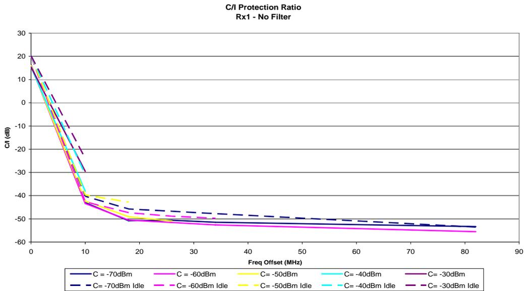
Figure 30: DTT Receiver 1 performance without filtering
