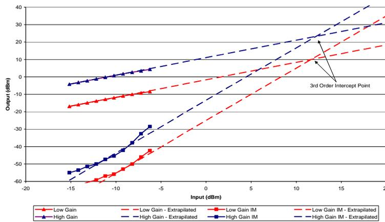
Figure 25: Amplifier 2 (masthead) 3<sup>rd</sup> order intercept point
