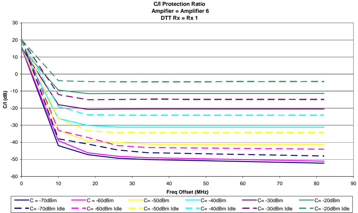
Figure 44: Amplifier 6 (indoor) with Rx1, without the use of filtering
