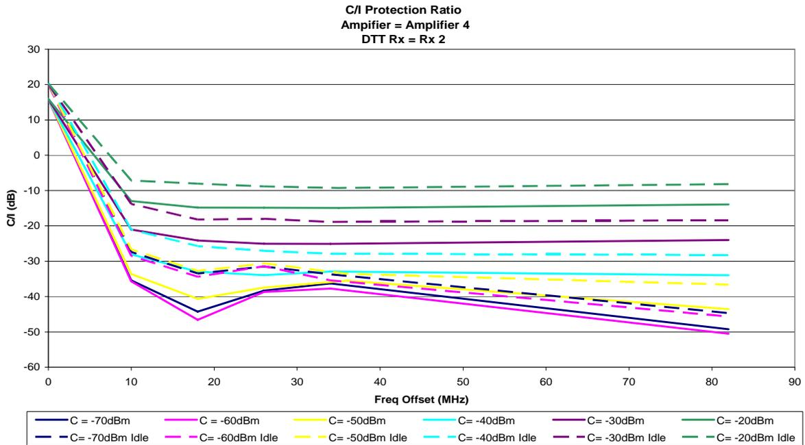
Figure 52: Amplifier 4 (indoor) with Rx2, without the use of filtering
