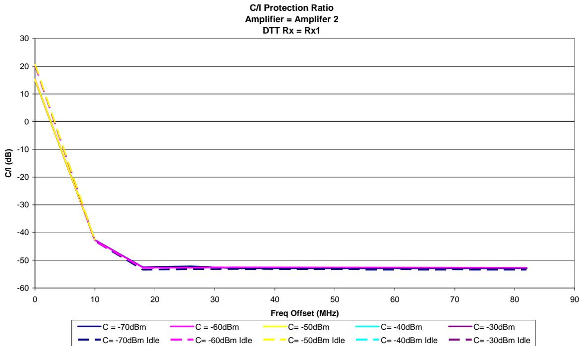
**Figure 37: Amplifier 2 (masthead) with Rx1, with filtering**
