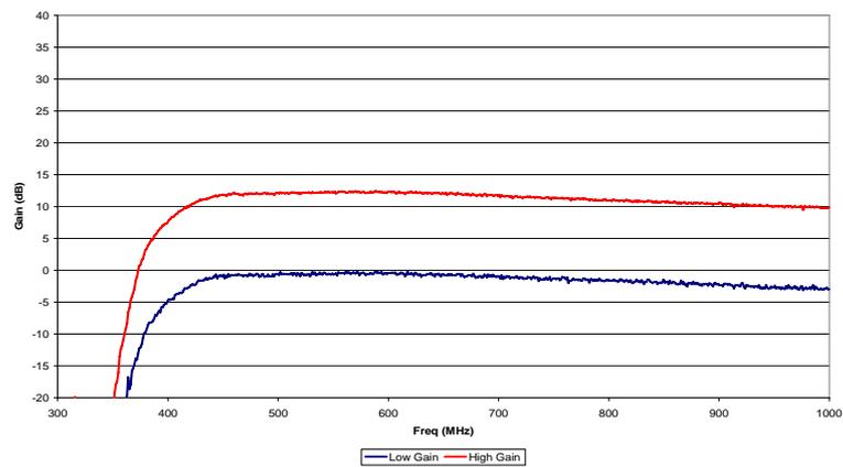
Figure 13: Amplifier 2 (masthead) gain response
