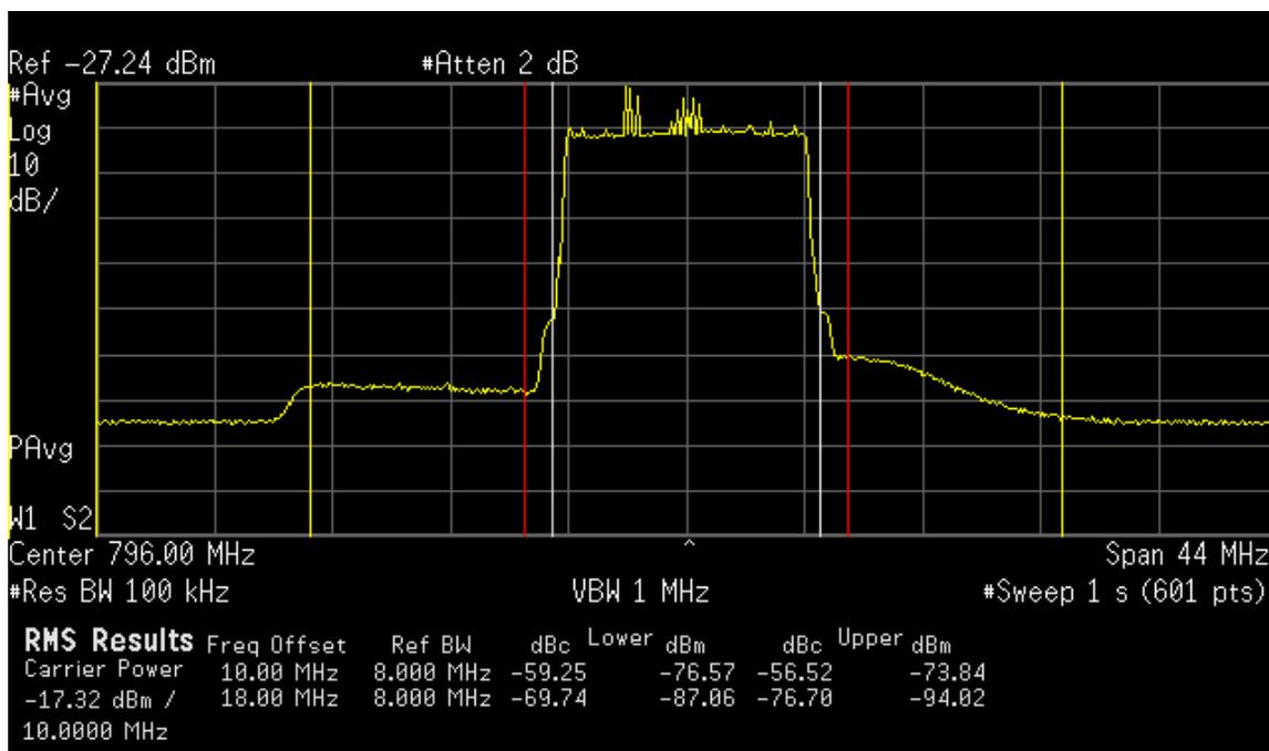
Figure 8: LTE base station emission under idle traffic conditions
