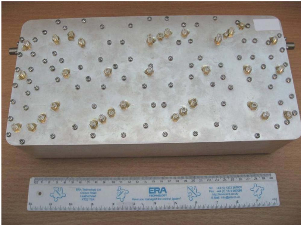
Figure 1: Prototype professional filter for use with masthead amplifiers
