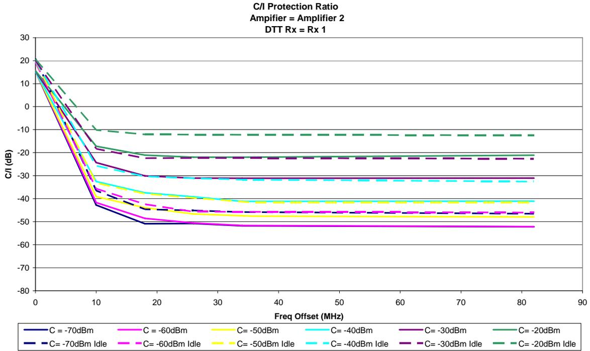
**Figure 36: Amplifier 2 (masthead) with Rx1, without the use of filtering**
