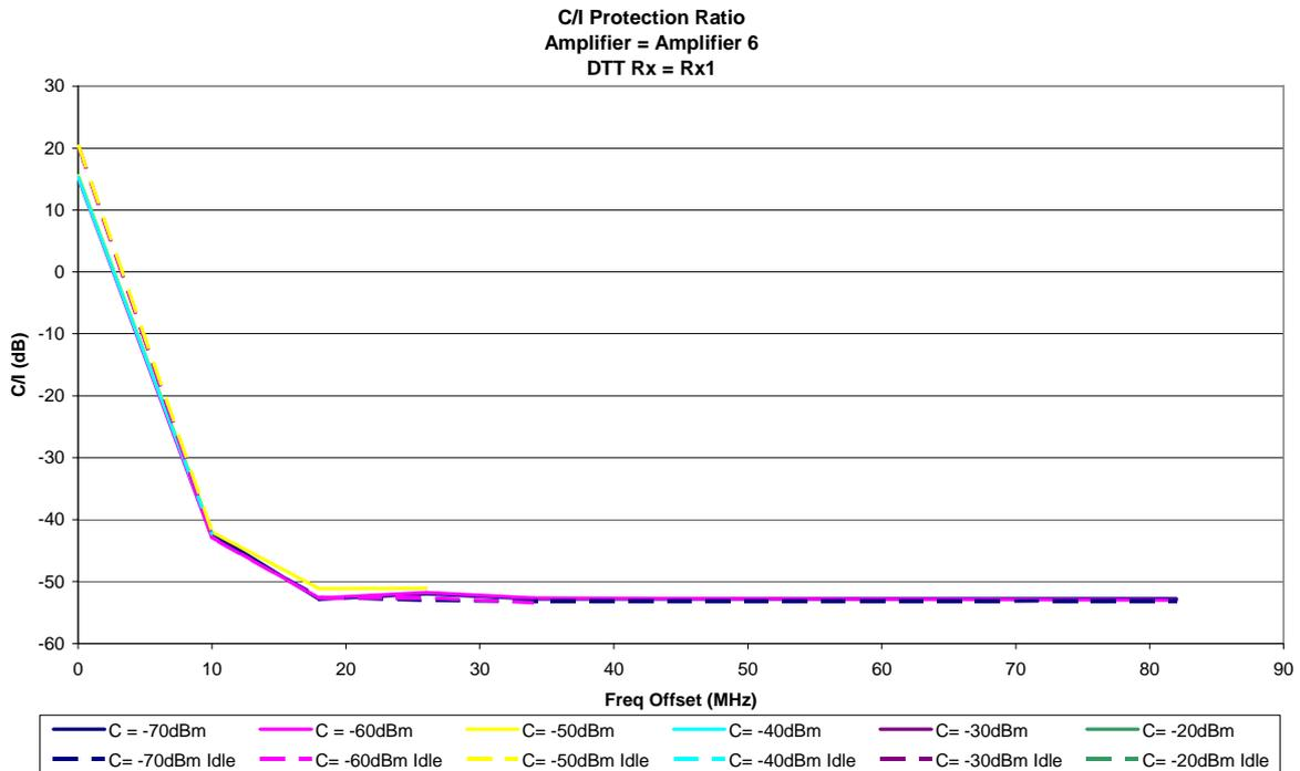
Figure 45: Amplifier 6 (indoor) with Rx1, with filtering
