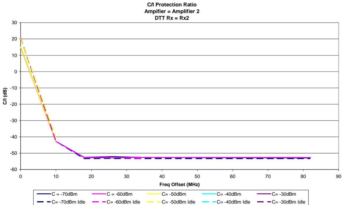
Figure 49: Amplifier 2 (masthead) with Rx2, with filtering
