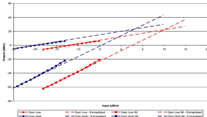
Figure 29: Amplifier 6 (indoor) 3<sup>rd</sup> order intercept point
