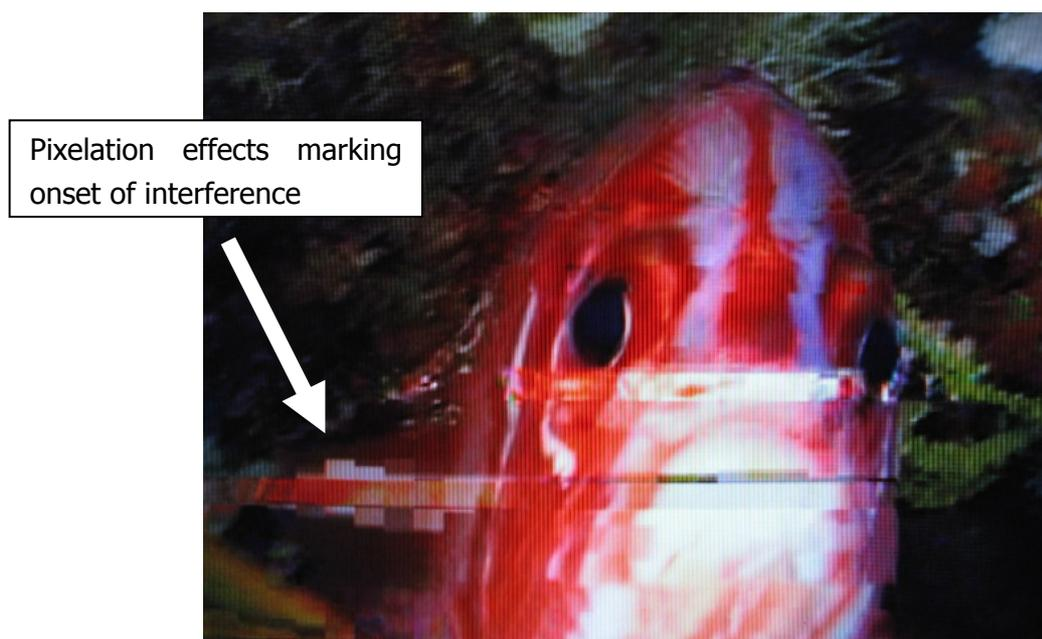
**Figure 10: Received picture showing onset of interference**
