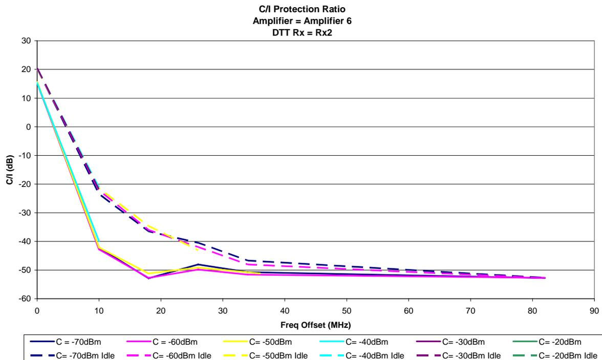
Figure 57: Amplifier 6 (indoor) with Rx2, with filtering
