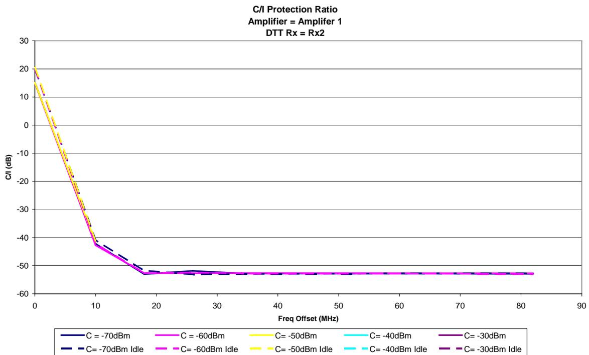
Figure 47: Amplifier 1 (masthead) with Rx2, with filtering
