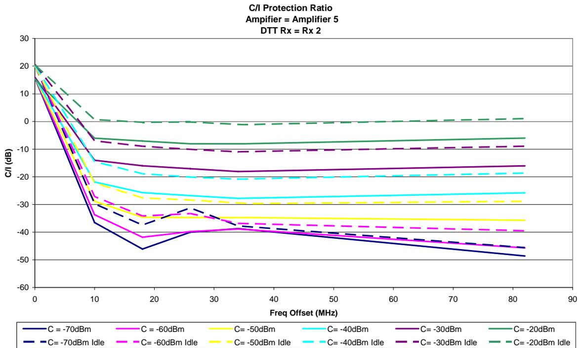
Figure 54: Amplifier 5 (indoor) with Rx2, without the use of filtering
