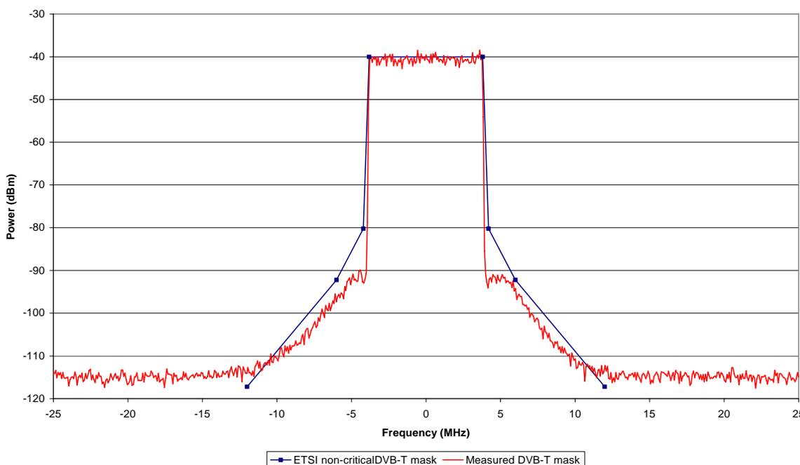
Figure 4: DVB-T wanted non-critical transmitter mask
