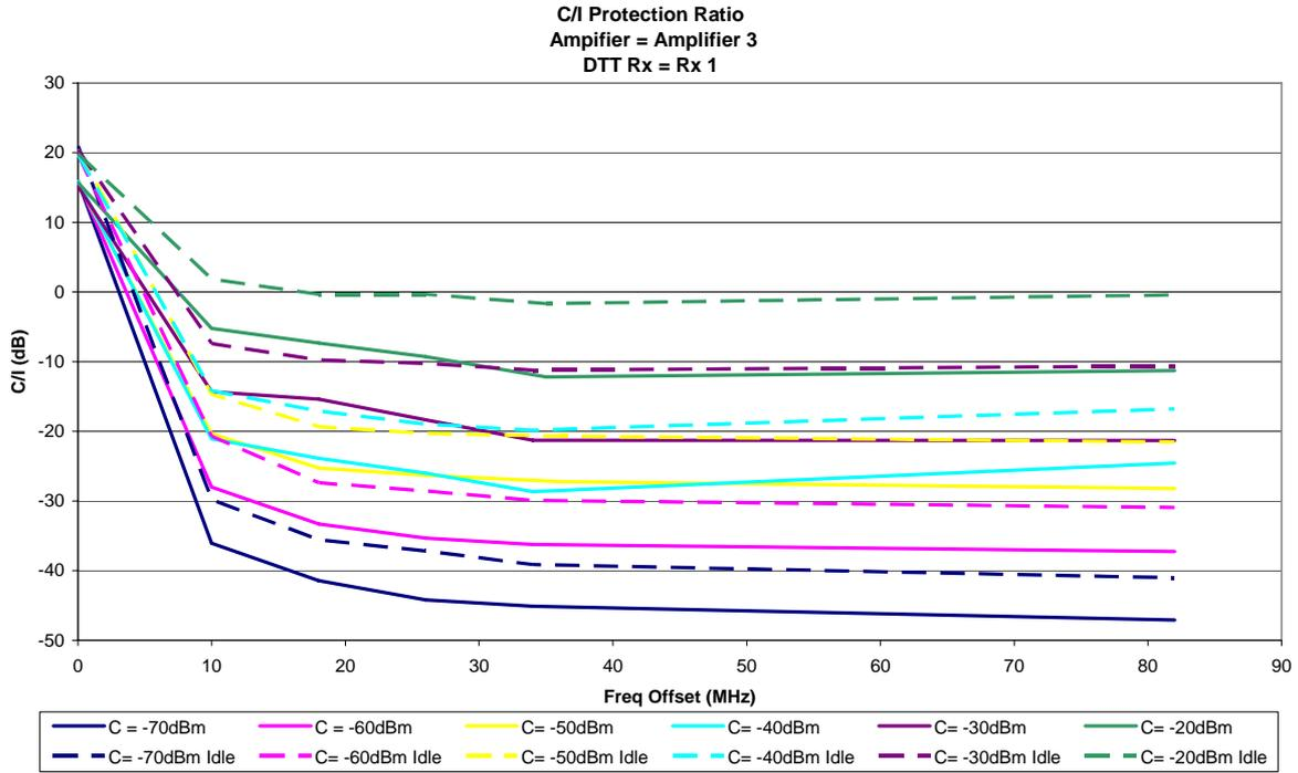
**Figure 38: Amplifier 3 (masthead) with Rx1, without the use of filtering**
