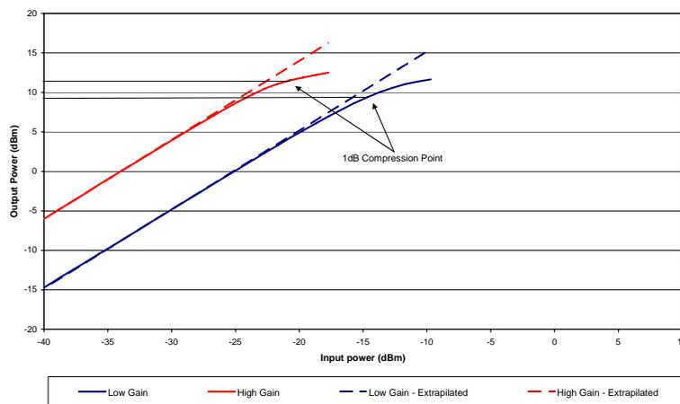
Figure 20: Amplifier 3 (masthead) 1 dB compression point
