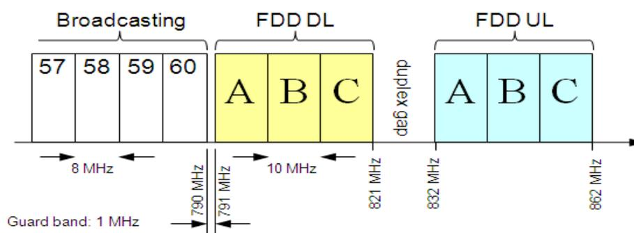
Figure 5: LTE and DTT Frequency Allocations
