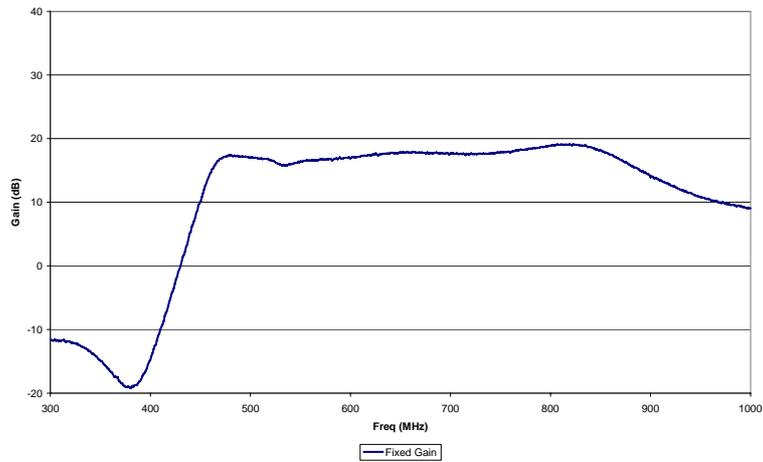
Figure 15: Amplifier 4 (indoor) gain response
