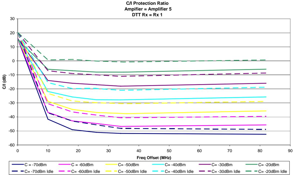
Figure 42: Amplifier 5 (indoor) with Rx1, without the use of filtering
