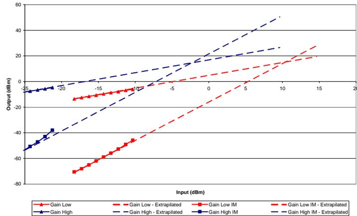
Figure 28: Amplifier 5 (indoor) 3<sup>rd</sup> order intercept point
