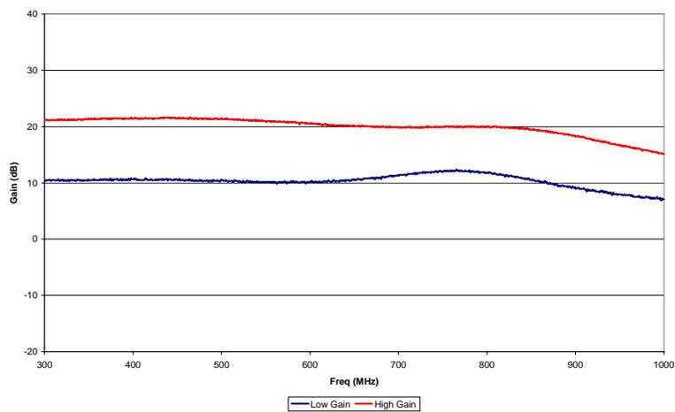
Figure 17: Amplifier 6 (indoor) gain response
