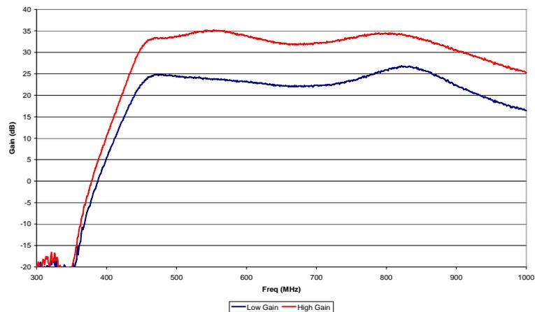
Figure 14: Amplifier 3 (masthead) gain response
