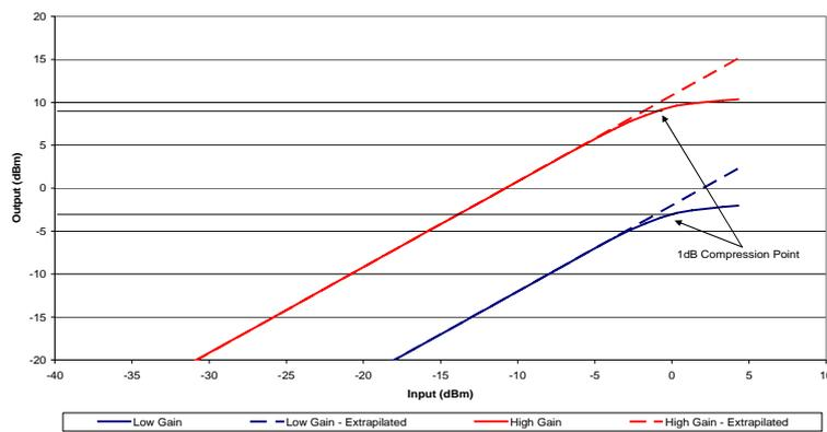
Figure 19: Amplifier 2 (masthead) 1 dB compression point
