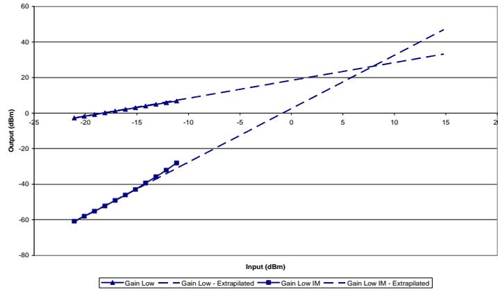
Figure 27: Amplifier 4 (indoor) 3<sup>rd</sup> order intercept point
