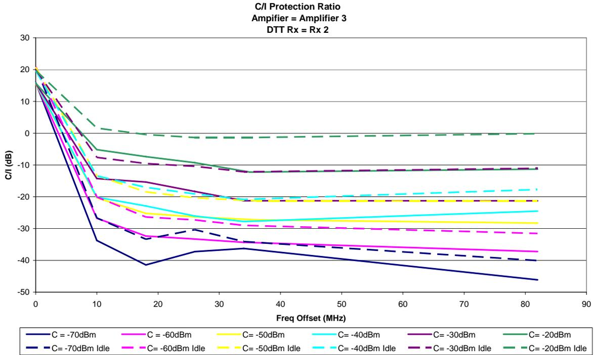
Figure 50: Amplifier 3 (masthead) with Rx2, without the use of filtering
