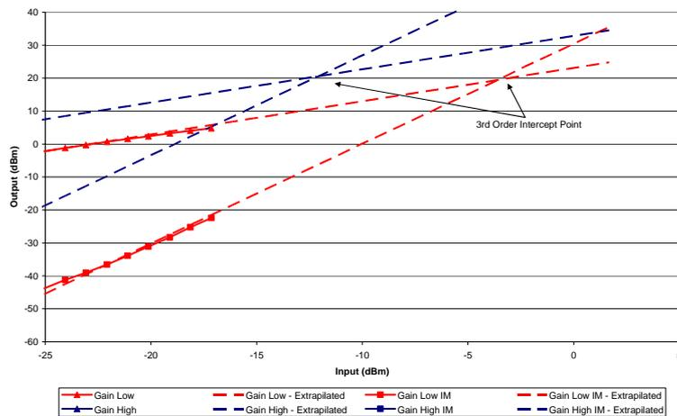
Figure 26: Amplifier 3 (masthead) 3<sup>rd</sup> order intercept point
