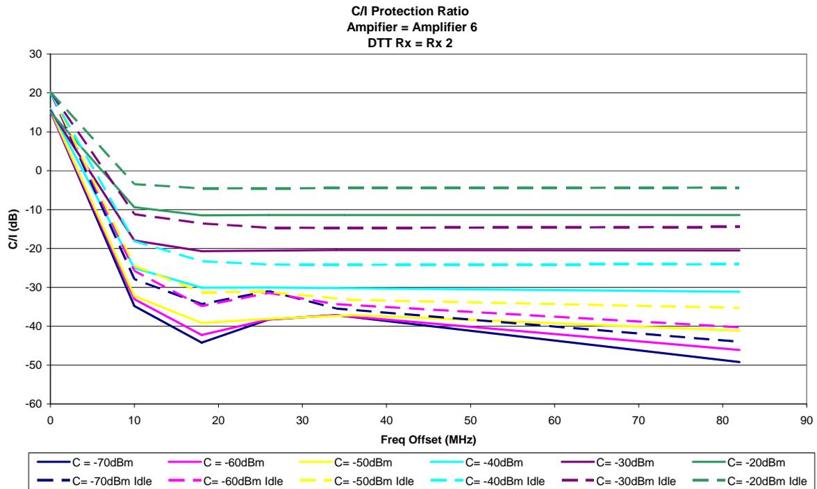
Figure 56: Amplifier 6 (indoor) with Rx2, without the use of filtering
