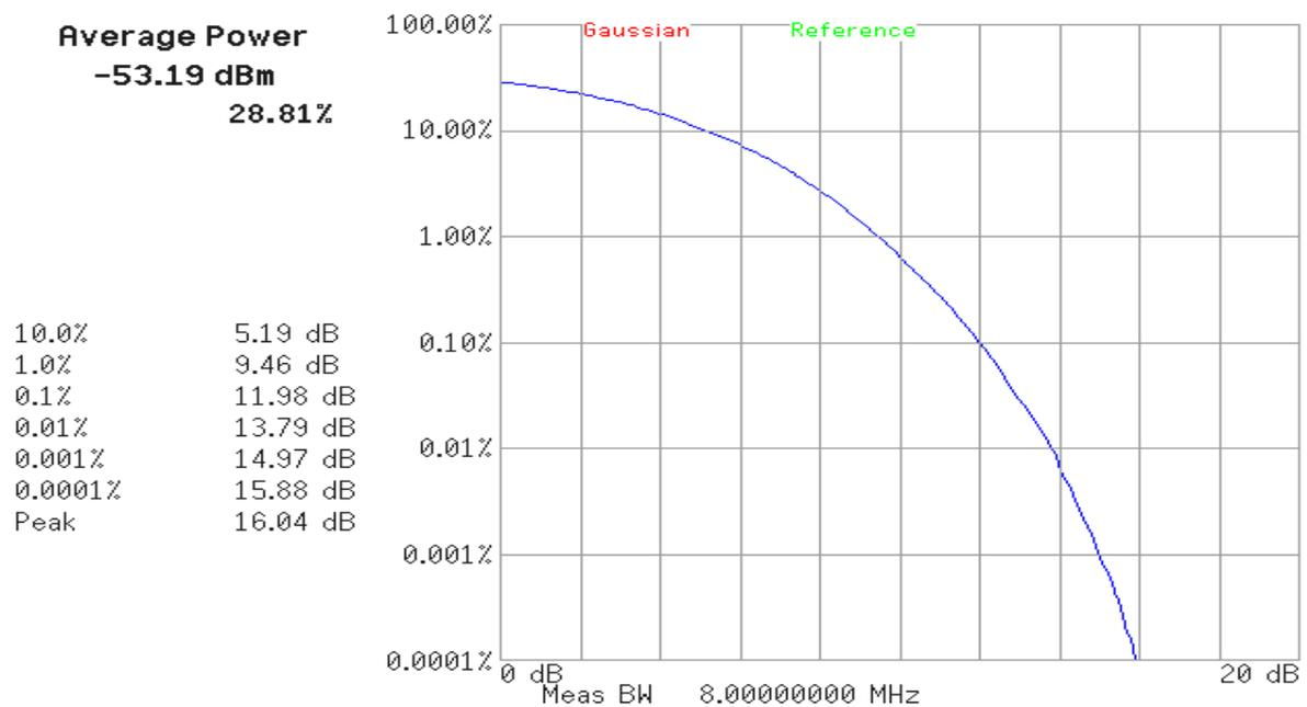
Figure 59: CCDF Measurement of LTE Idle Signal
