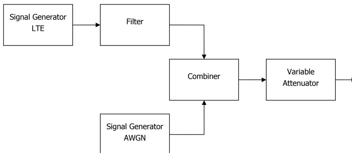
Figure 6: Generation of LTE base station interferer
