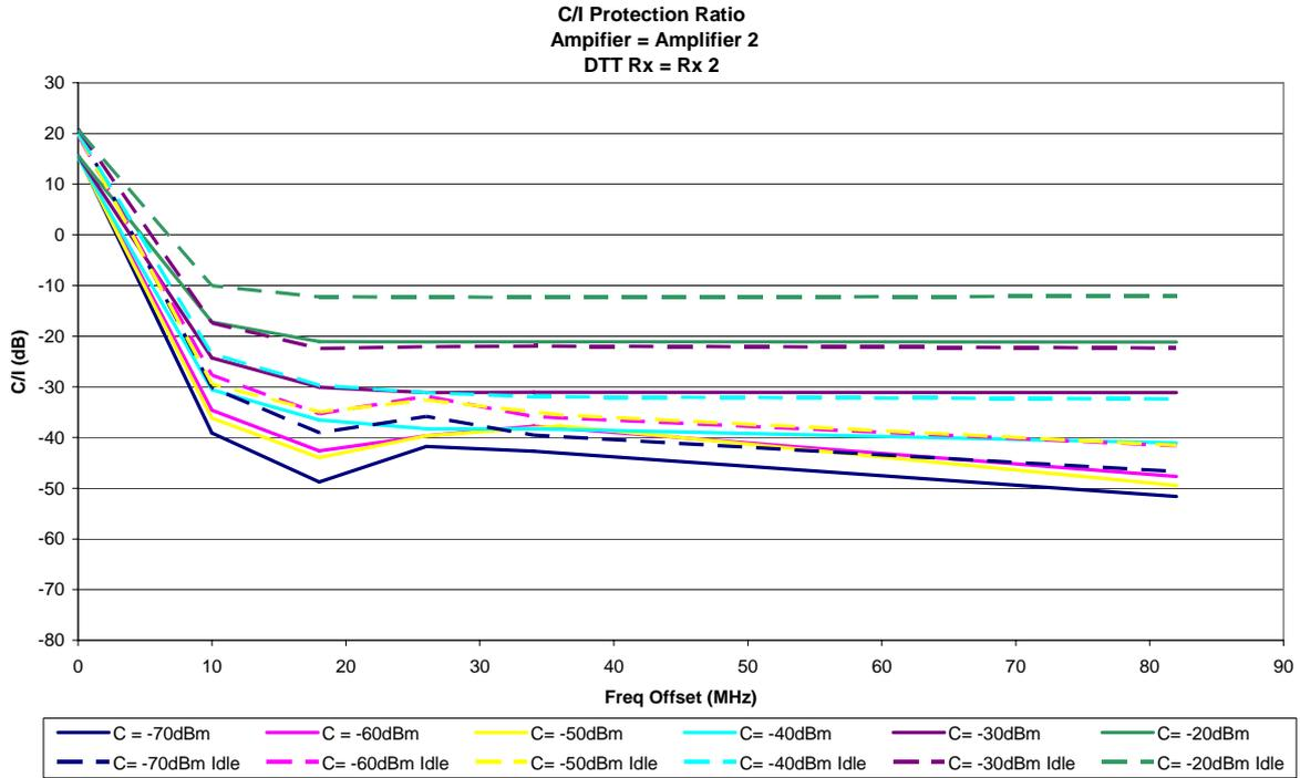
Figure 48: Amplifier 2 (masthead) with Rx2, without the use of filtering
