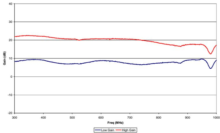
Figure 16: Amplifier 5 (indoor) gain response
