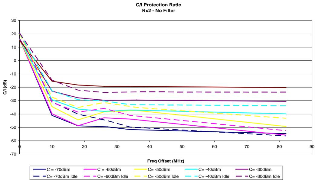
**Figure 32: DTT Receiver 2 performance without filtering**
